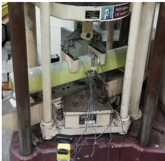
Figure 5: The leading edge demonstrator installed for a 4-point bending test in the Denison 500 test machine at NUI Galway
