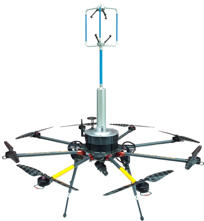
Figure 1: Measurement system WindLocator (unfolded) without battery packs
