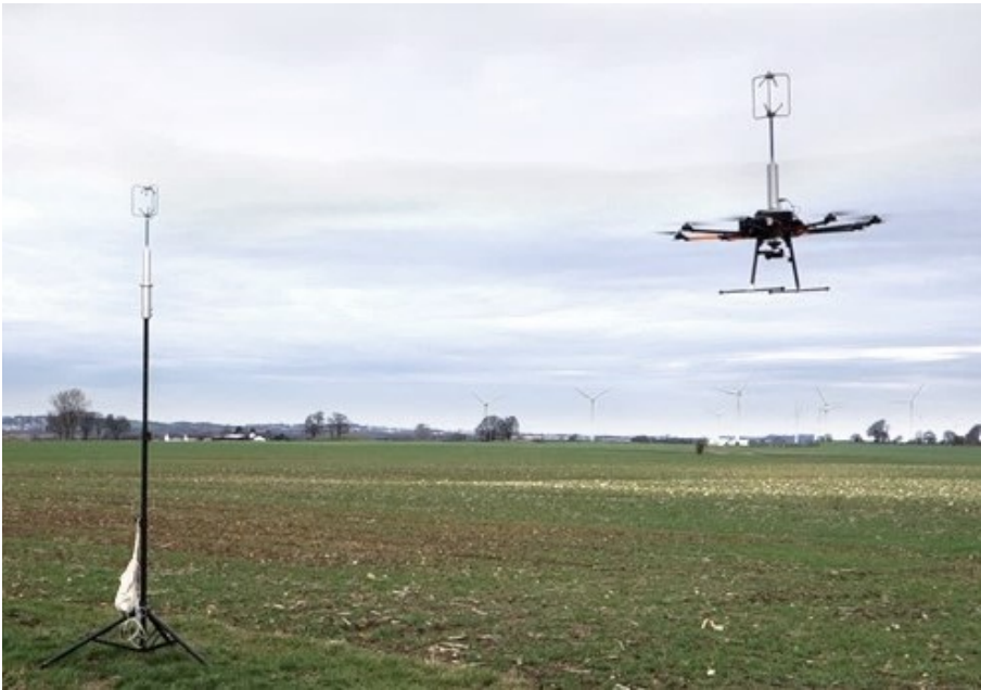
Figure 5 WindLocator hovering close to stationary anemometer
