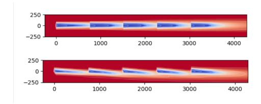
**Figure 7.** Flow field of 5 turbines using GCH for the baseline case (top) and the optimized case (bottom). The optimized yaw angles are based on the values shown in Table 1.
