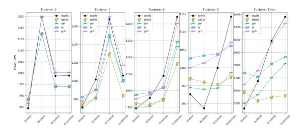
**Figure 10.** Absolute power values for each turbine (excluding the upstream turbine) in the five turbine array for a wind speed of 8 m/s and high turbulence, i.e., 10% turbulence intensity. Total turbine power is shown in the far right plot. The x-axis shows the combination of yaw angles plotted.
