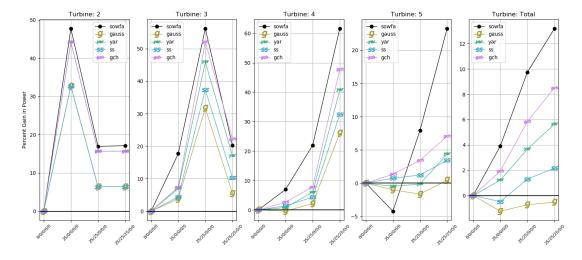
**Figure 11.** Power gains for each turbine (excluding the upstream turbine) in the five turbine array for a wind speed of 8 m/s and high turbulence, i.e., 10% turbulence intensity. Total power gain is shown in the far right plot. The x-axis shows the combination of yaw angles plotted.
