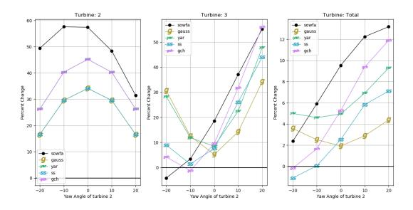
Figure 5. Comparison of changes in power when sweeping the angle of the second turbine, i.e. Turbine 2, when the angle of the first turbine, i.e., Turbine 1 is set to  $+20^{\circ}$  where the wind speed was 8 m/s and the turbulence intensity was 6%. The results of the change in power of the third turbine, as well as the overall total of all three turbines, reflect the importance that the two yaw offsets are in the same direction.
