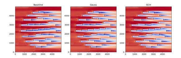
**Figure 12.** Flow field results from SOWFA where the wind direction is 270° (Case 2). The left plot shows the baseline case with all turbines aligned with the flow. The middle plot shows the flow field with yaw angles from the optimized Gaussian model and the right plot shows the flow field with the yaw angles from the optimized GCH model.
