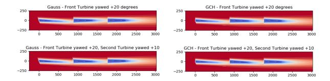
**Figure 4.** FLORIS results for the three-turbine case shown for the Gaussian model (left) and the GCH model (right), where the first turbine is yawed  $20^{\circ}$  (top row) and the first turbine is yawed  $20^{\circ}$  and the second turbine is yawed  $10^{\circ}$  (bottom row).
