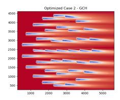
**Figure 14.** Flow fields of the optimized Gaussian model (left) and the optimized GCH model (right) for Case 2 where the wind direction is at  $270^{\circ}$ .
