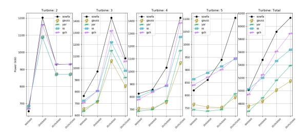
**Figure 8.** Absolute power values for each turbine (excluding the upstream turbine 1) in the five turbine array for a wind speed of 8 m/s and low turbulence, i.e., 6% turbulence intensity. Total turbine power is shown in the far right plot. The x-axis shows the combination of yaw angles plotted.
