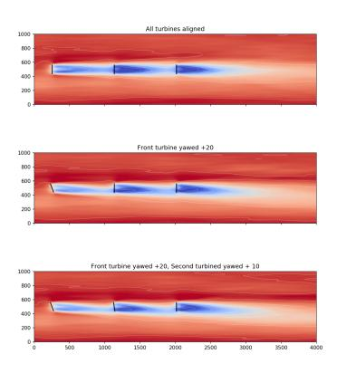
Figure 3. Three-turbine array in SOWFA where all turbines are aligned (top), the first turbine is yawed  $+20^{\circ}$  (middle), and the first turbine is yawed  $+20^{\circ}$  and the second turbine is yawed  $+10^{\circ}$ .
