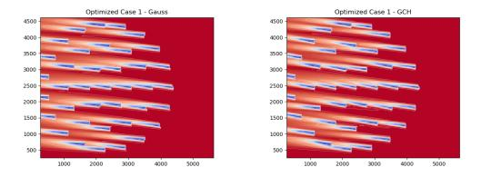
**Figure 13.** Flow fields of the optimized Gaussian model (left) and the optimized GCH model (right) for Case 1 where the wind direction is at 95°.
