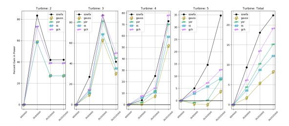
**Figure 9.** Power gains for each turbine (excluding the upstream turbine 0) in the five turbine array for a wind speed of 8 m/s and low turbulence, i.e., 6% turbulence intensity. Total power gain is shown in the far right plot. The *x*-axis shows the combination of yaw angles plotted.
