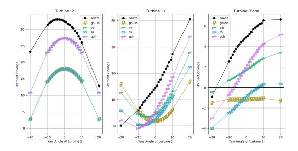
Figure 6. Comparison of changes in power when sweeping the angle of the second turbine, i.e. Turbine 2, when the angle of the first turbine, i.e., Turbine 1 is set to  $+20^{\circ}$  where the wind speed was 8 m/s and the turbulence intensity was 10%.
