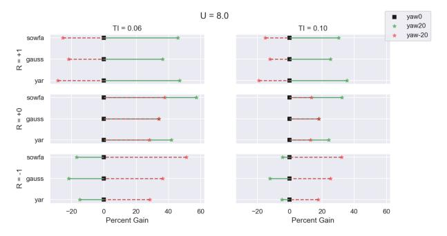
**Figure 2.** Results for percent change of power in the second turbine in each offset location, for each of model, at 8 m/s and 6% turbulence intensity (left) and 10% turbulence intensity (right). The results are shown where the second turbine is offset +R (top row), 0R (middle row), and -R (bottom row).
