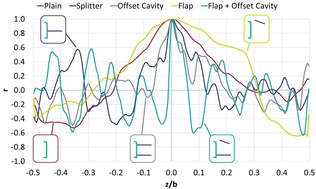
*Figure 1. Pearson correlation coefficient of the lift coefficient ( $C_l$ ) time-series with respect with the midsection (placed at  $z/b=0$ ) for the various configurations. High positive values indicate strong positive correlation and highly negative values suggest a strong negative correlation.*
