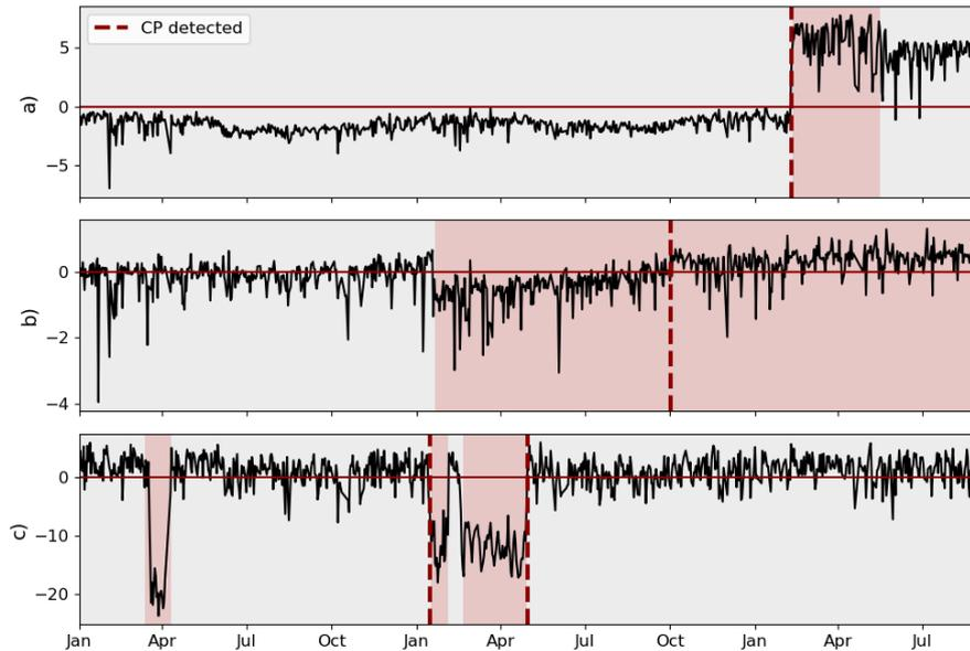
**Figure 11.** Examples of partially correct classified oil temperature (a), gearbox bearing temperature (b) and pitch motor winding temperature (c). Each change in background color indicates a true CP, each dashed line indicates a detected CP.
