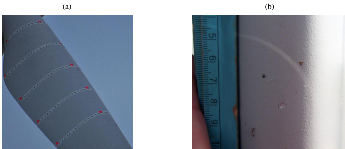
Figure 1. Rotor blades of utility scale wind turbines (a) Flow indicators to detect early separation in the root region, reproduced and modified from Pechlivanoglou et al. (2013). (b) Leading edge roughness, reproduced and modified from Pechlivanoglou et al. (2010).
