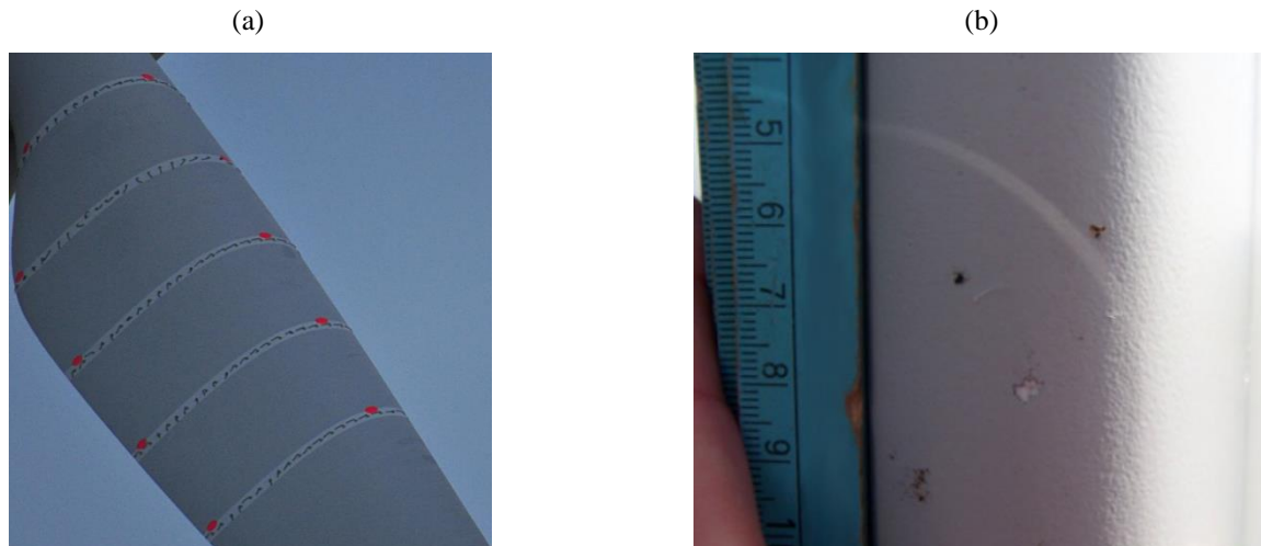
35 Figure 1. Rotor blades of utility scale wind turbines (a) Flow indicators to detect early separation in the inner blade region, reproduced from Pechlivanoglou et al. (2013). (b) Leading edge roughness, reproduced from Pechlivanoglou et al. (2010).
