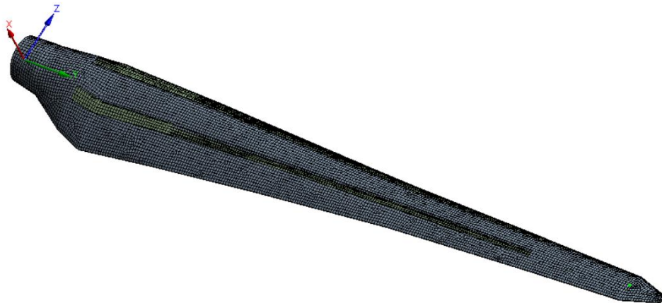
Figure R 6. Location of the deflection measurement point.
