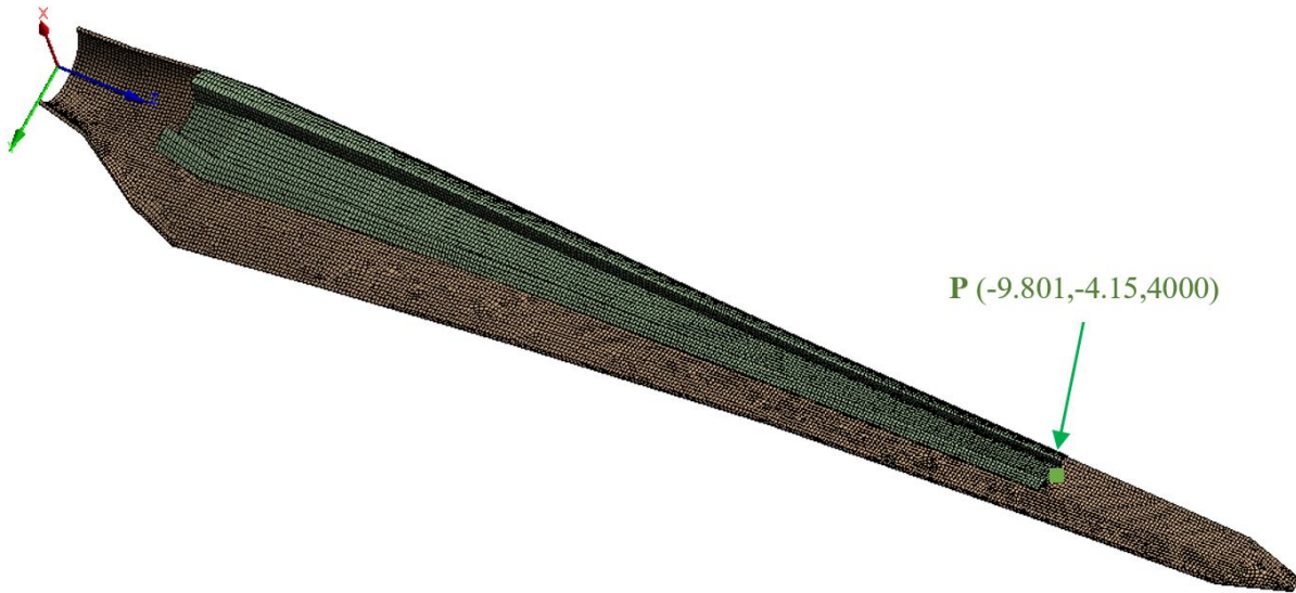
Figure 6. Location of the load measurement coordinate system and the deflection measurement point P.
