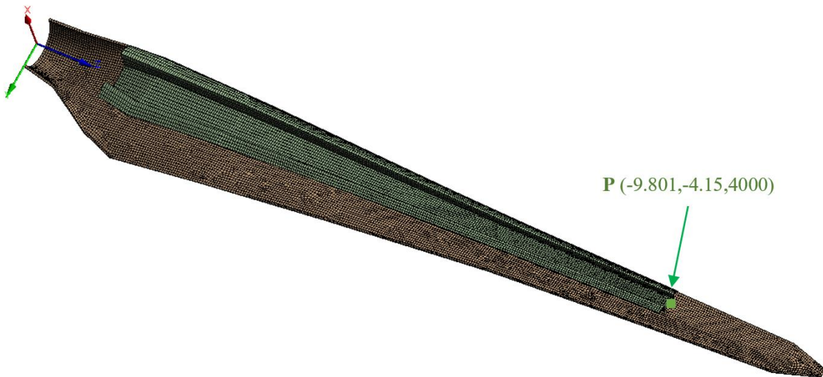
205 Figure 6. Location of the load measurement coordinate system and the deflection measurement point P.
