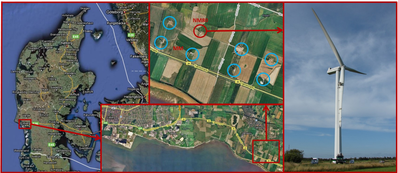
Figure 1. Map of the site approx. 10 km south-east of Esbjerg (© Google Maps 2007). The test turbine, NM80 is situated in a small wind farm at Tjæreborg along with 7 other wind turbines of size around 2 MW. The other turbines are circled with blue and the test turbine is marked by the red circle. The meteorology mast is shown by the 'MM' denotation in the picture.
