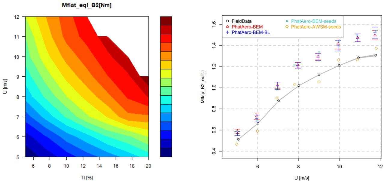
(a) Field data variation with wind speed  $U$  and turbulence intensity  $TI$  (b) Comparison between field data and simulations at  $TI=10\%$  as a function of wind speed (all values are non-dimensionalized using the average of the field data results over the wind speed bins)
