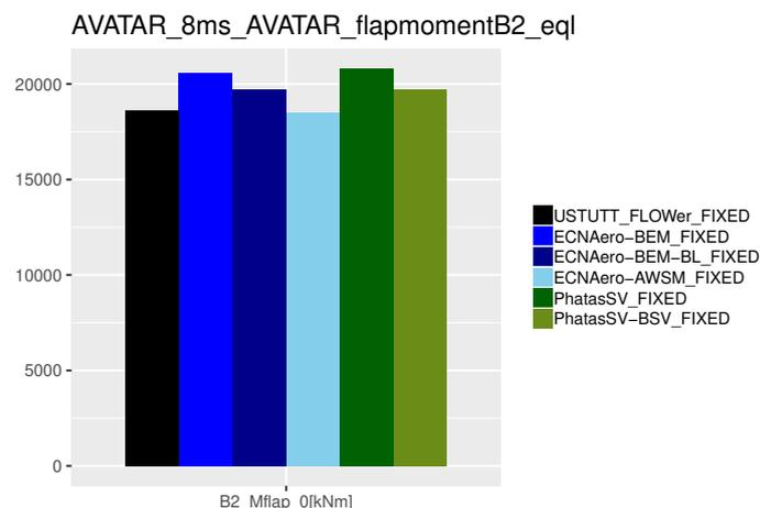
**Figure 5.** Effect of shed vorticity modeling on fatigue equivalent flapwise blade root moment ( $U_{\infty}=8$  m/s fixed)
