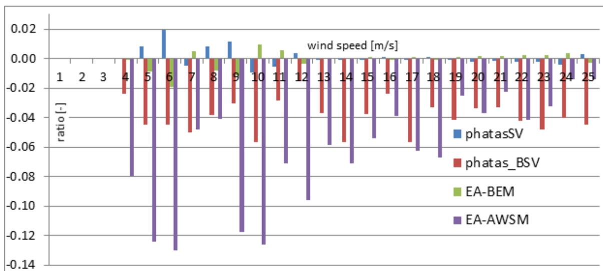
560 **Figure 11.** Ratio of blade root flap fatigue loading relative to the average of phatasSV and PhatAero(EA)-BEM as a function of wind speed featuring higher axial induction factors, in agreement with the observations from section 2 for the comparison to CFD. For wind velocities above rated the fatigue predictions with blade shed vorticity model (Phatas-BSV) are close to the AWSM vortex wake simulations.
