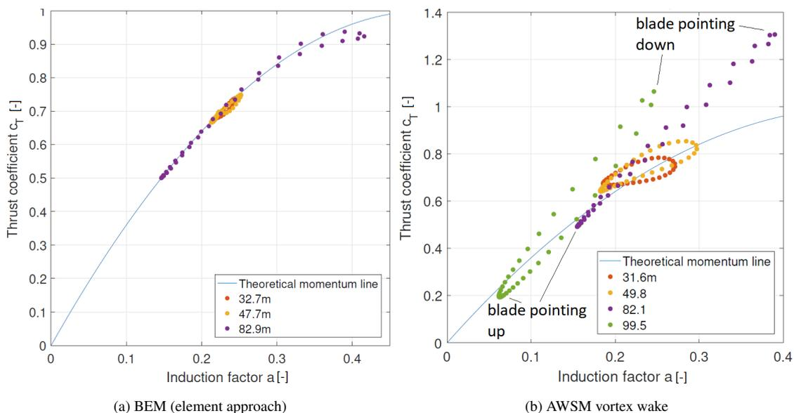
**Figure 6.** Comparison of post-processed AVATAR rotor simulation results in heavy shear ( $U=8$  m/s,  $\alpha = 0.75$ ) for several radial stations against the theoretical momentum line
