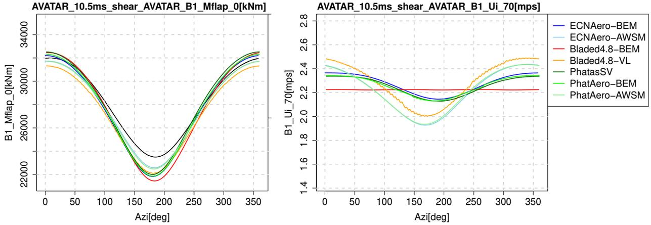
(a) Azimuthal variation of flapwise blade root moment Mflap
