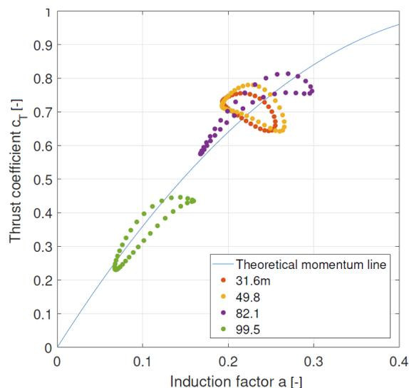
**Figure 7.** Comparison of post-processed AVATAR rotor simulation results in heavy shear (AWSM vortex wake,  $U=8$  m/s,  $\alpha = 0.75$ ) for several radial stations against the theoretical momentum line. The reference wind speed for non-dimensionalizing  $C_t$  and  $a$  is now taken as the sector averaged wind speed
