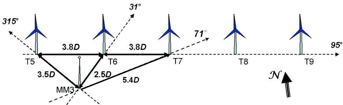
**Figure 9.** Main dimensions and directions in the EWTW farm. T5 to T9 are the turbine positions, MM3 indicates the measurement mast. Dimensions are expressed in rotor diameters D.
