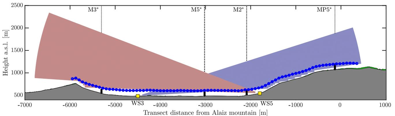
**Figure 4.** Transect scan on the vertical plane spanned by WS3 and WS5 (yellow squares). Shaded areas represent the superimposed RHI scans after a hard target filtering. The blue dots show the transect scan measured by WS2 and WS4 (out of the plane). The black dots indicate the positions of the masts M3, M5, M2 and MP5 when projected onto the transect's plane.
