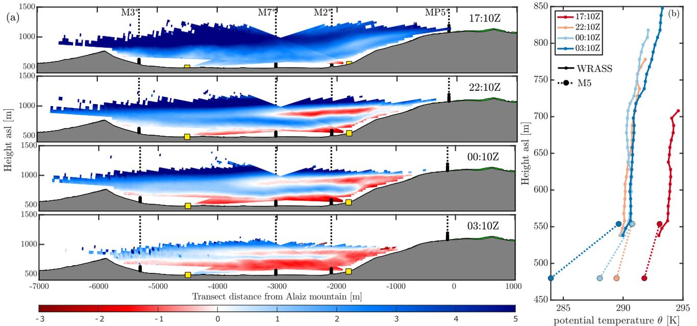
**Figure 12.** Panel (a) shows the superposition of dual RHI scans during the layered valley winds period between 24<sup>th</sup>–25<sup>th</sup> October 2018. Panel (b) shows the potential temperature profiles measured by the sodar RASS and M5 at each frame in (a).
