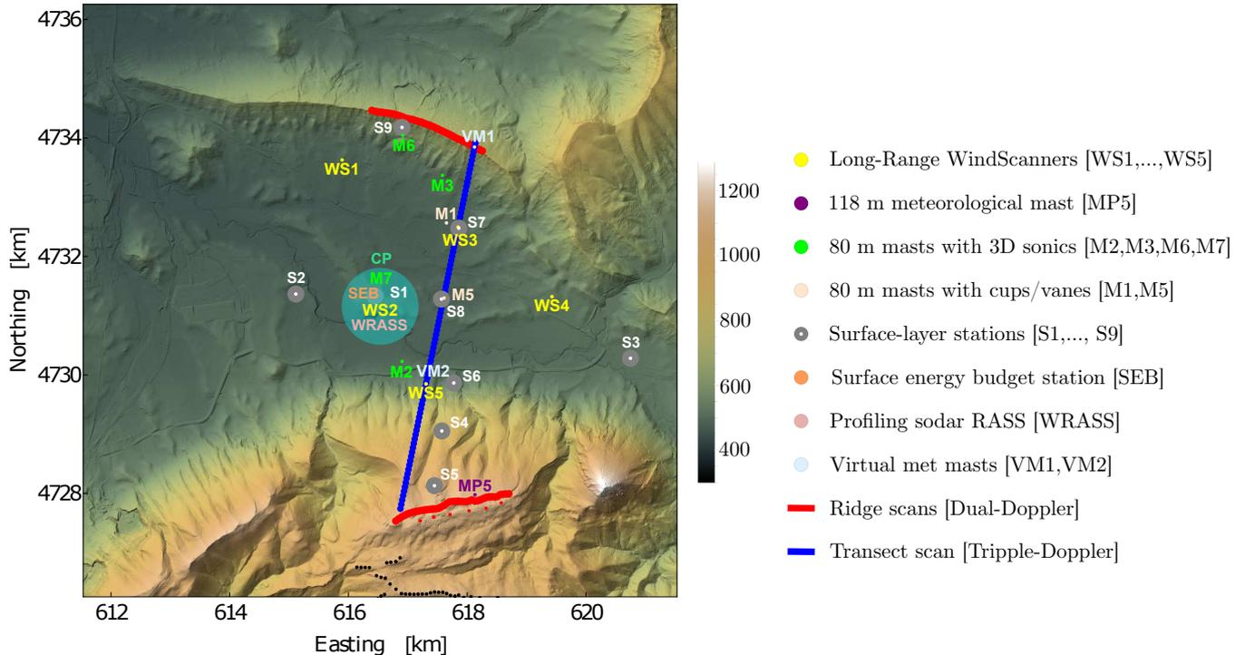
**Figure 3.** Instrumentation layout of the ALEX17 campaign within the 10 x 10 km experimental domain centered at CP. The legend details each type of measurement station. The transect scan (blue line), detailed in figure 4, is the focus of this study.
