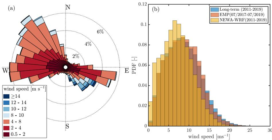
**Figure 6.** Panel (a) shows the wind rose of 10-min wind speeds at the valley measured by M5 at 80 m agl. Panel (b) shows the wind speed distributions at 118 m agl measured at MP5 during the reference period and EMP along with the modeled wind speeds from NEWA-WRF for the reference period.
