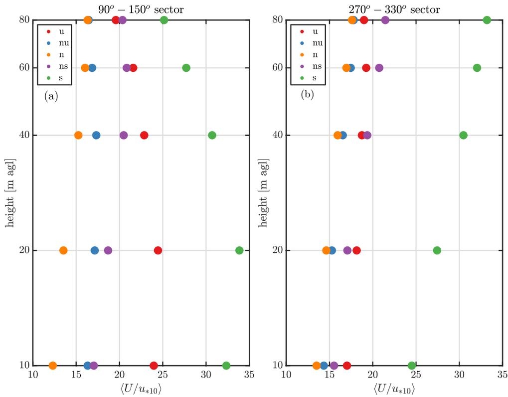
**Figure 8.** Mean vertical wind profiles normalized with the friction velocity computed by the 10-min sonic anemometer ( $u_{*10}$ ). Panel (a) shows profiles within the  $120^\circ \pm 30^\circ$  sector and panel (b) shows profiles within the  $300^\circ \pm 30^\circ$  sector based on wind directions at 10m.
