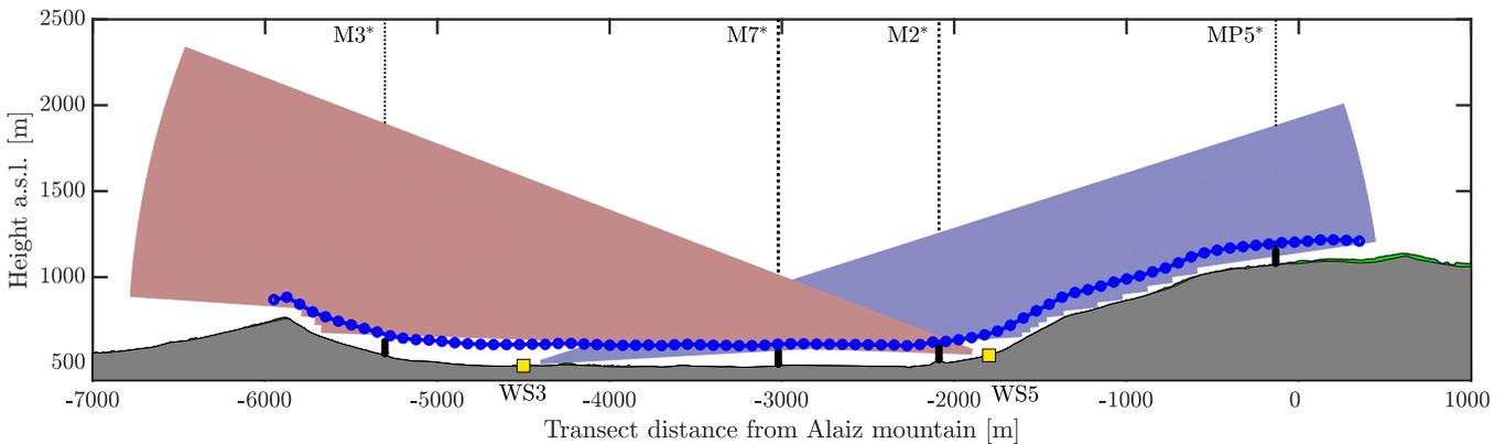
**Figure 4.** Transect scan on the vertical plane spanned by WS3 and WS5 (yellow squares). Shaded areas represent the superimposed RHI scans after a hard target filtering. The blue dots show the transect scan measured by WS2 and WS4 (out of the plane). The black dots indicate the positions of the masts M3, M7, M2 and MP5 when projected onto the transect's plane.
