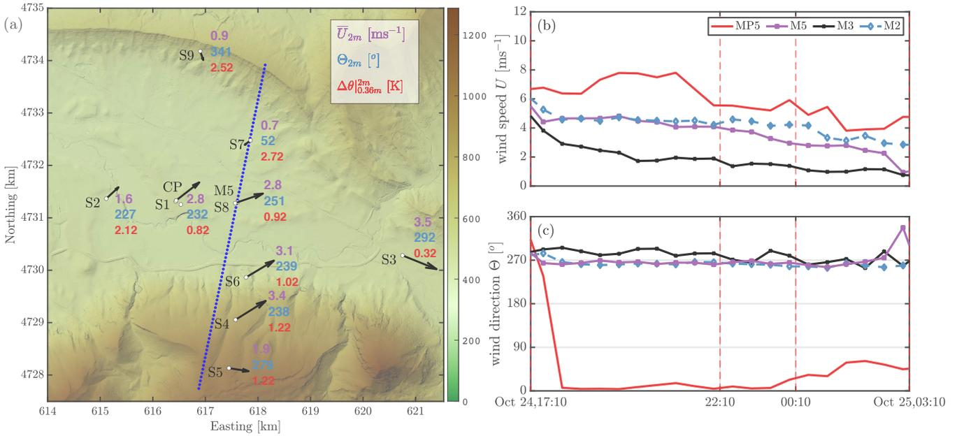
**Figure 13.** Panel (a) shows surface layer stations’ wind and potential temperature measurements at 24-10-2018 22:30Z. Panels (b) and (c) show the time series of wind speed and direction from the masts, respectively. The vertical dashed lines represent the snapshots of figure 12.
