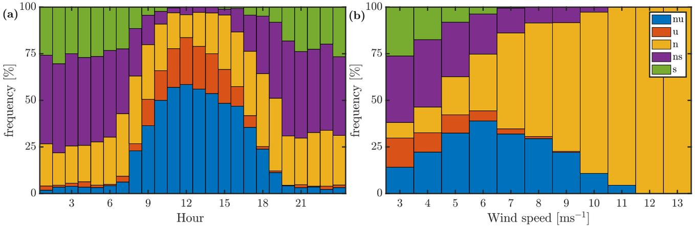
**Figure 7.** Frequency of  $z/L$  at 10 m agl divided in stability classes per hour (a) and per wind speed (b) from measurements at M7. The stability classes are found in table 2.
