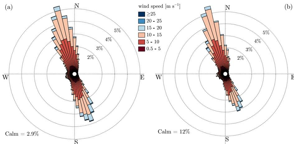
**Figure 5.** Wind roses of 10-min wind speeds observed by MP5 at 118 m for the reference period (2011–2019) (a) and during the EMP (b). The calm threshold is  $0.5 \text{ m s}^{-1}$ .
