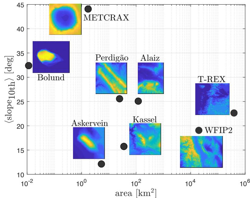
**Figure 1.** Illustration of the complexity of some atmospheric flow experiments as a function of their area of coverage. The complexity is in terms of the slope: the average 10<sup>th</sup> percentile of the highest slopes. The inserts besides the markers show contour maps of the relative elevation for each site.
