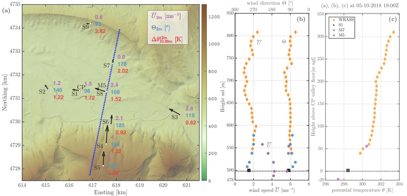
**Figure 11.** Wind conditions during hydraulic jump case at 05-10-2018 19:00Z. Panel (a) shows surface-layer stations’ wind and potential temperature measurements. Panels (b) and (c) show vertical profiles of wind and potential temperature at the valley from the sodar RASS, M7, S1 and M5. The dashed line marks the valley floor level at CP.
