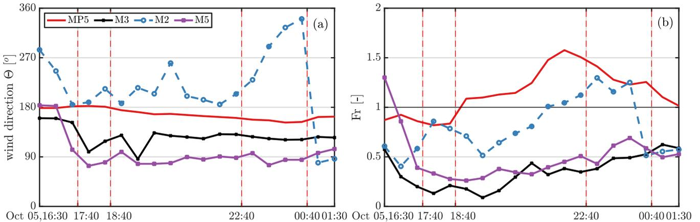
**Figure 10.** Time series of wind direction (a) and Froude number (b) during the hydraulic jump case. The vertical dashed lines represent the snapshots of figure 9.
