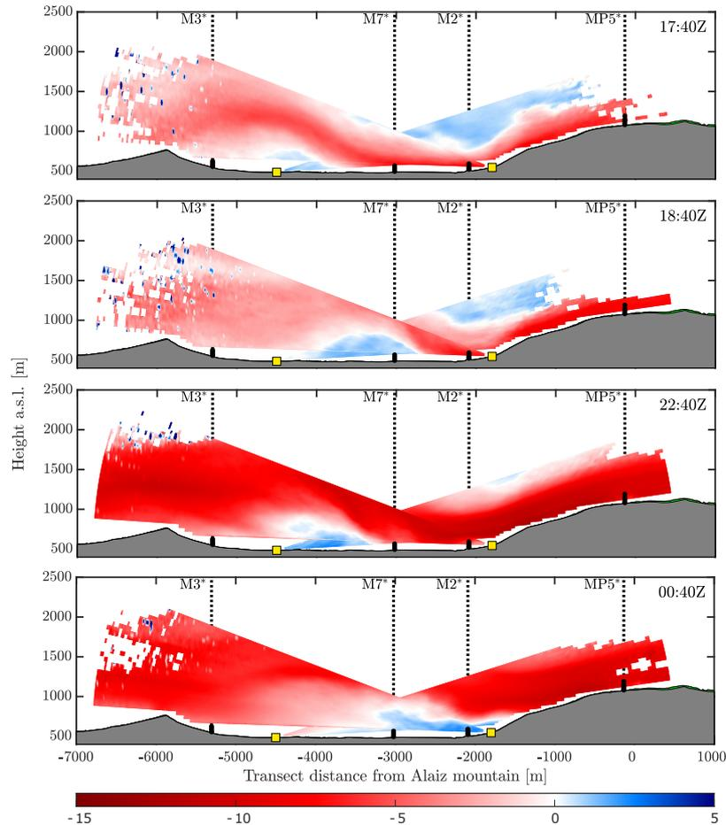
**Figure 9.** Superposition of dual RHI scans during the hydraulic jump period between 5<sup>th</sup>–6<sup>th</sup> October 2018. The color bar represents radial wind speed in  $\text{ms}^{-1}$  with negative values representing flow from right to left. Each of the frames correspond to a 10-min scan.
