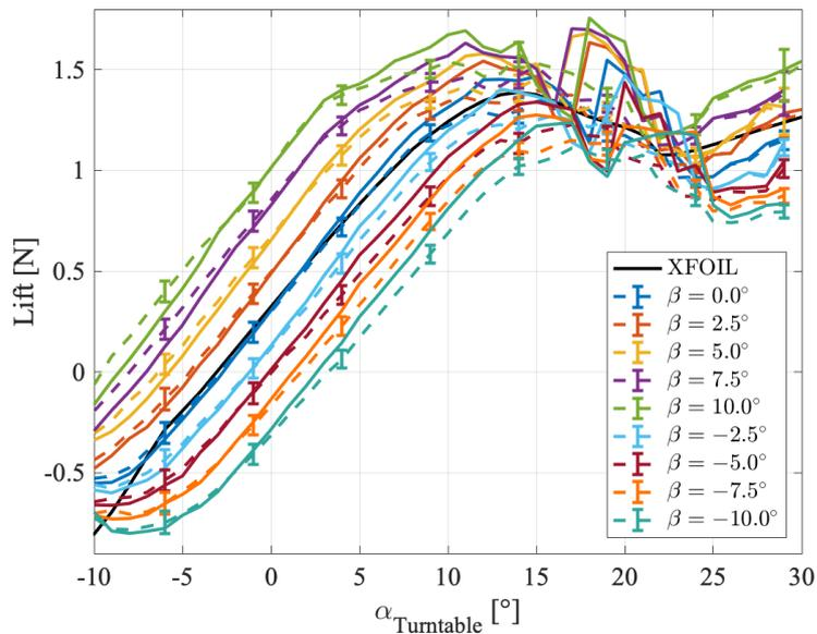
Figure 3 Lift comparison between balance measurements (dashed lines) and full pressure port integration (solid lines). Additionally XFOIL result for beta = 0° is shown.
