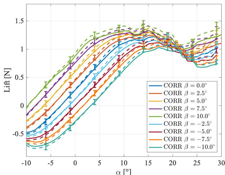
Figure 1 Comparison between uncorrected balance measurements (dashed lines) and blockage corrected results (solid lines).
