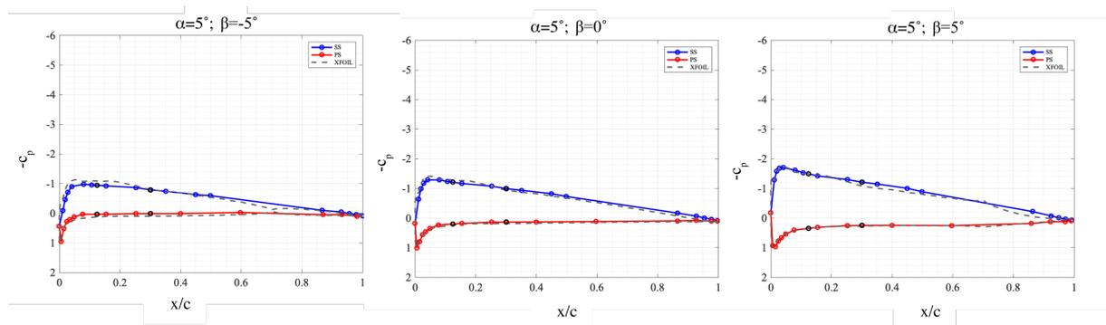
Figure 2 Comparison of measured  $c_p$  distributions to XFOIL calculations. Exemplary  $\alpha=5^\circ$  for three flap angles ( $-5^\circ, 0^\circ, 5^\circ$ ) are shown.
