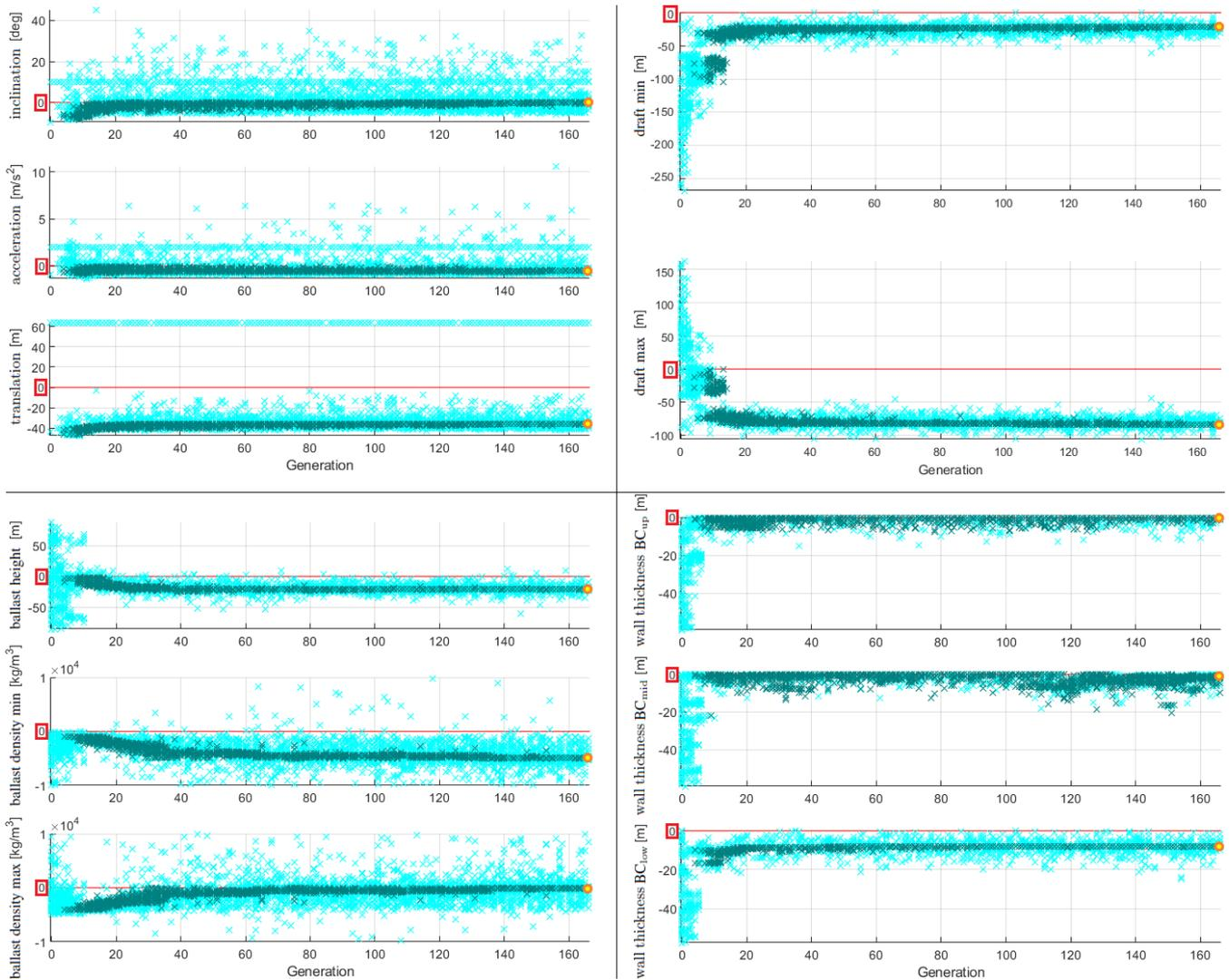
**Figure 4.** Development of the constraints within the iterative optimization process; all simulated individuals are represented by light cyan crosses and those complying with all constraints by dark bluish green crosses, the best-performing individual is marked with a yellow filled circle framed in orange, and the value corresponding to the reference FOWT system is plotted as a red line.
