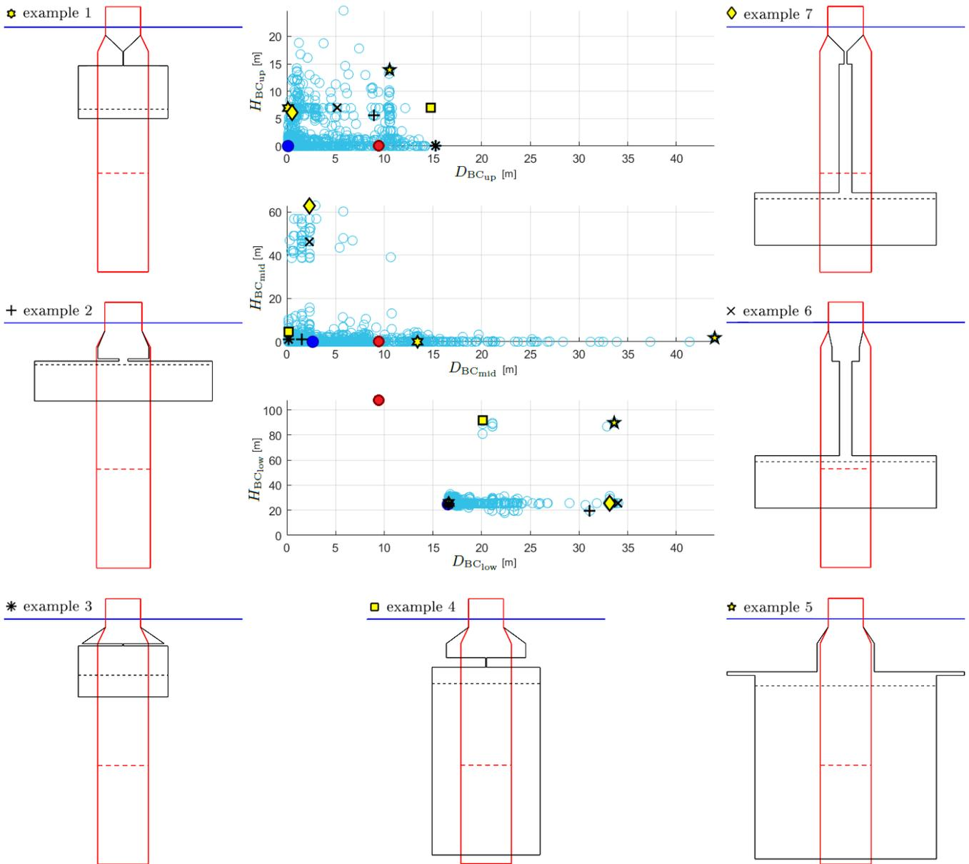
**Figure 5.** Exemplary potential innovative floater geometries selected from the individuals complying with all constraints; the individuals complying with all constraints are represented by unfilled light blue circles, the best-performing individual is marked with a dark blue filled circle, and the value corresponding to the reference FOWT system is plotted as a red filled circle with the associated shape drawn with a red line.
