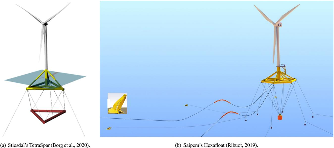
**Figure 6.** Pendulum-stabilized innovative floating platform concepts.
