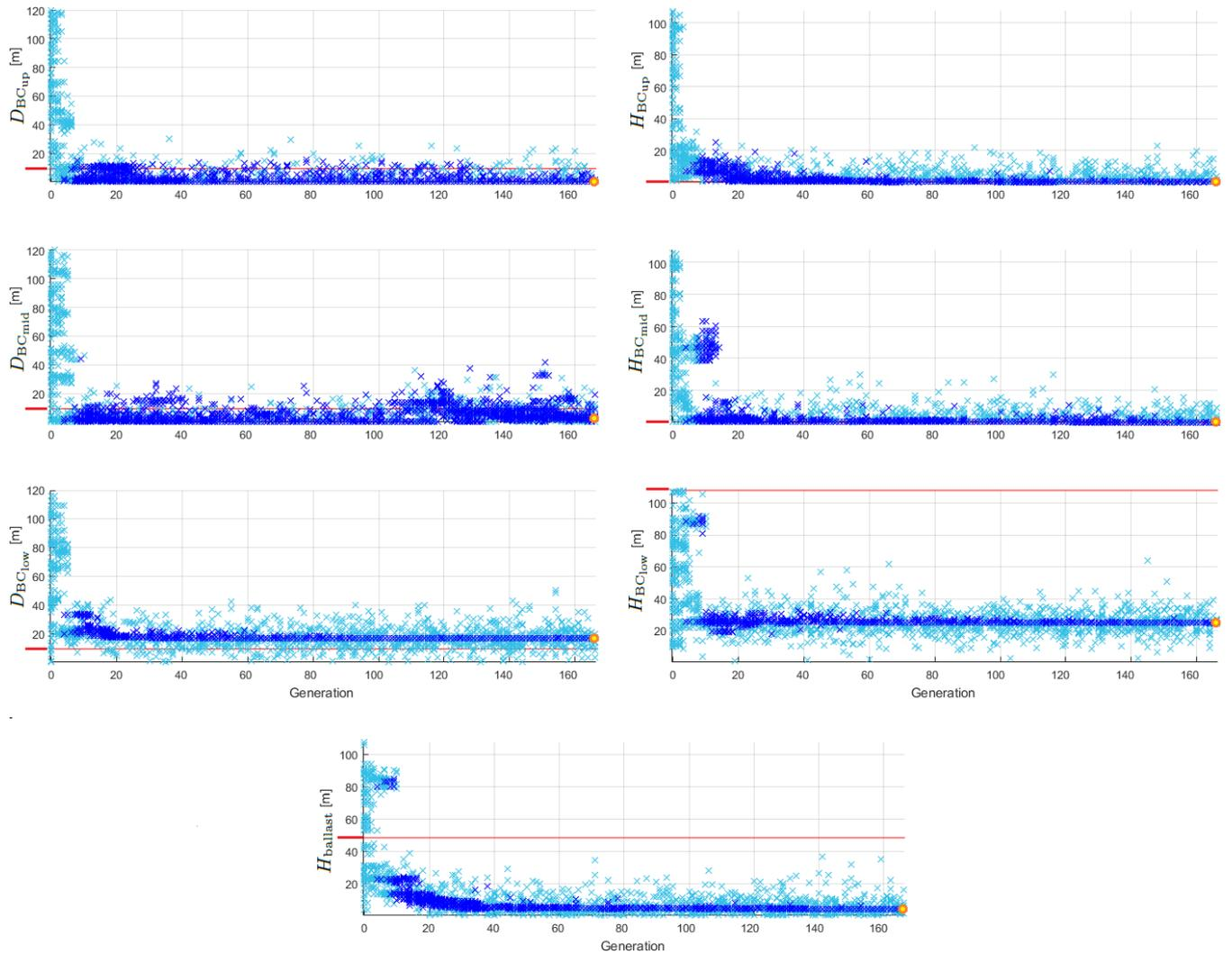
**Figure 3.** Development of the design variables within the iterative optimization process; all simulated individuals are represented by light blue crosses and those complying with all constraints by dark blue crosses, the best-performing individual is marked with a yellow filled circle framed in orange, and the value corresponding to the reference FOWT system is plotted as a red line.
