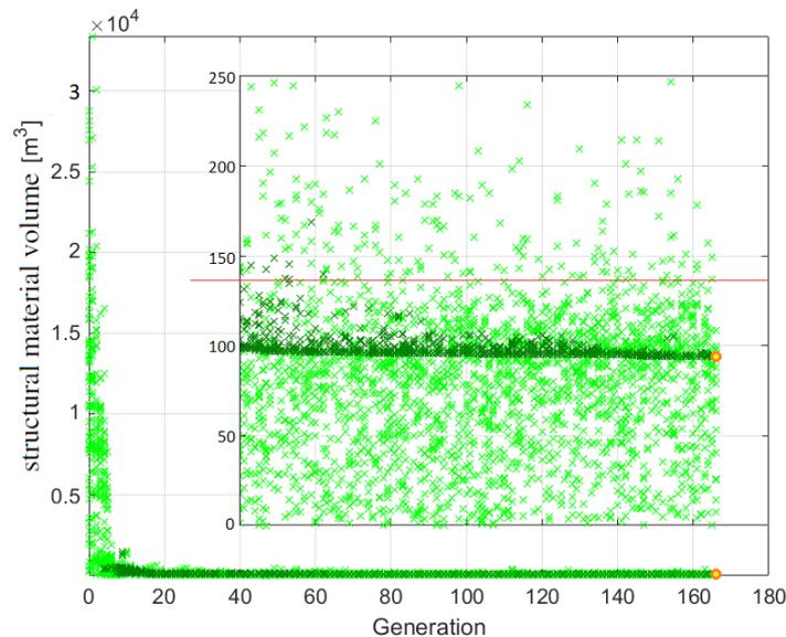
**Figure 7.** Development of the objective function within the iterative optimization process; all simulated individuals are represented by light green crosses and those complying with all constraints by dark green crosses, the best-performing individual is marked with a yellow filled circle framed in orange, and the value corresponding to the reference FOWT system is plotted as a red line.
