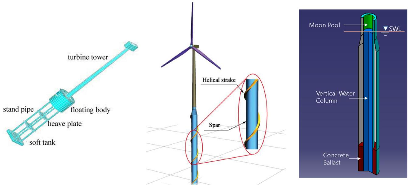
(a) Truss spar-type platform (Chen et al., 2017).
