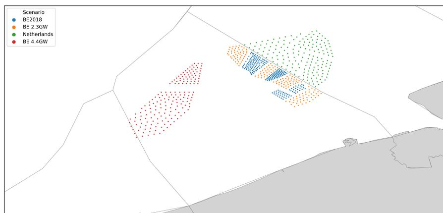
**Figure 3.** Plant and turbine locations for the different stages of offshore wind installations. The Dutch plants are taken into account when modelling external wake impacts on the Belgian fleet
