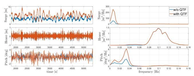
Figure 16. Activefloat response to EWM 50 years wind and ESS
