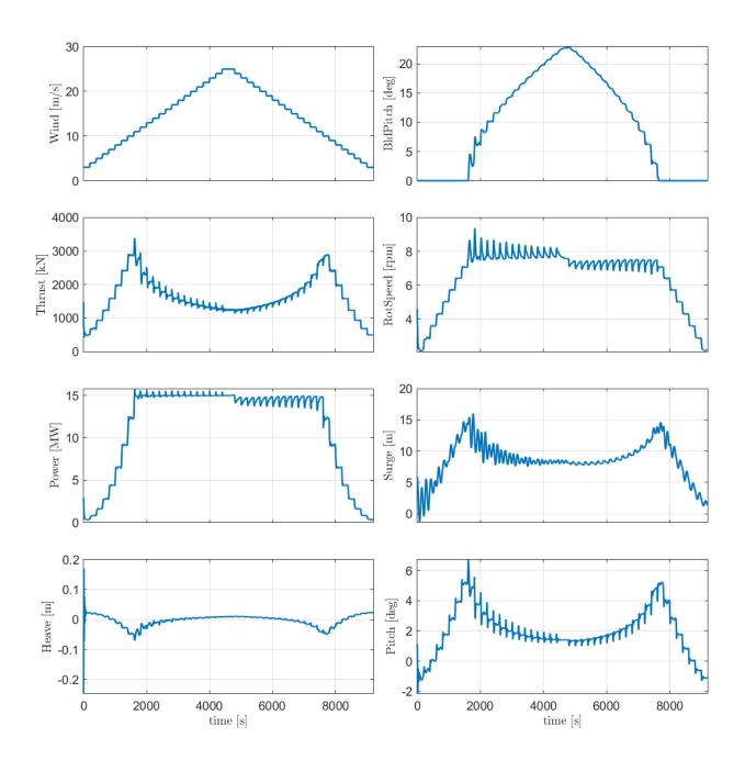
Figure A1. Activefloat response to step wind in absence of waves
