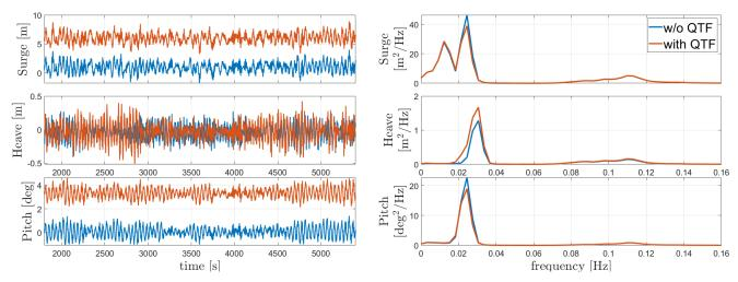
Figure 15. WindCrete response to EWM 50 years wind and ESS
