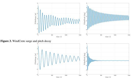
Figure 4. Activefloat surge and pitch decay
