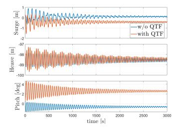
Figure 8. WindCrete response to regular waves at CG
