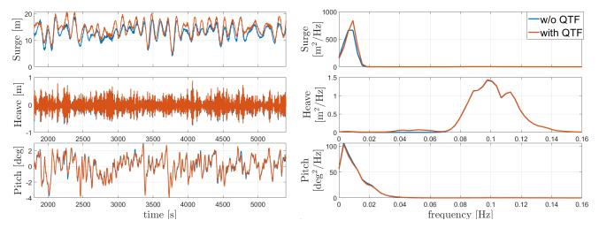
Figure 12. Activefloat response to NTM wind and ESS
