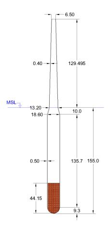
Figure 1. WindCrete geometry (units in meter)
