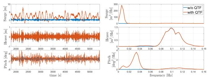
Figure 10. Activefloat response to irregular waves in absence of wind
