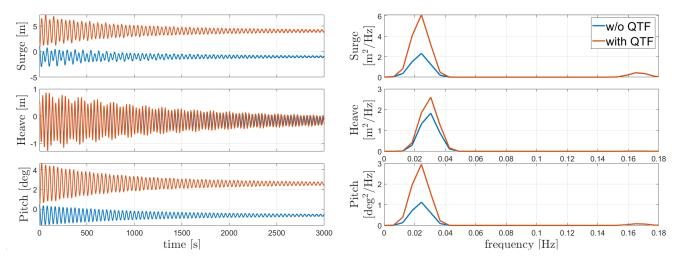
Figure 6. WindCrete's response to regular waves without and with second order forces
