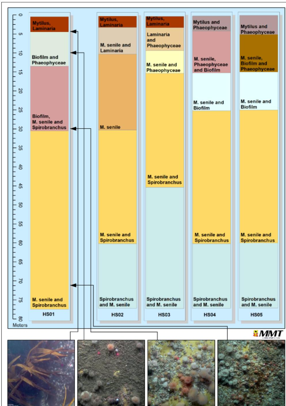
Figure 6 Illustration of faunal zonation at Turbine Substructure HS01 – HS05. Order of taxa indicates dominance, with dominant taxa listed first.
