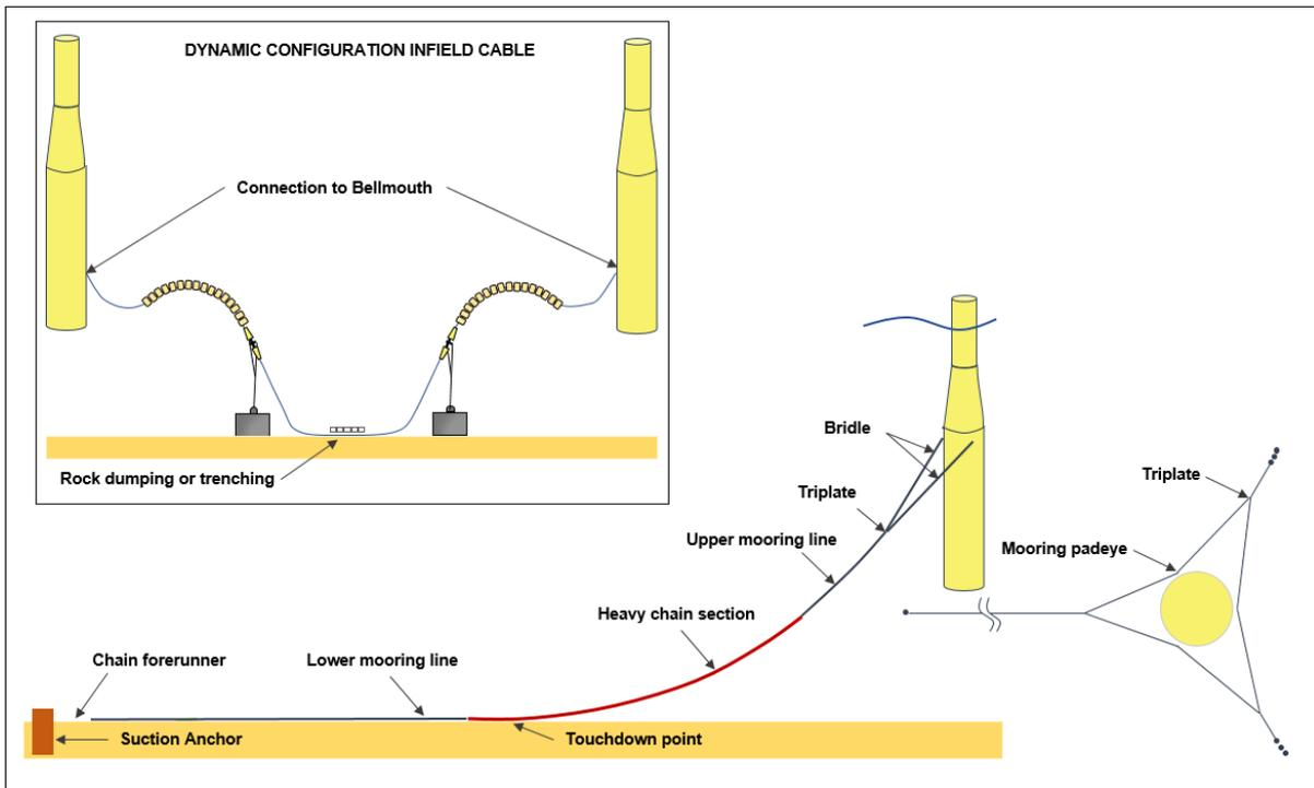
95 **Figure 2 Layout of Turbine Substructures, Mooring Lines, Suction Anchors and Infield Cables. Figure based on schematic provided by Equinor.**
