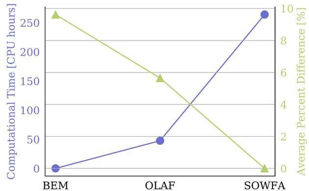
**Figure 9.** Computational time and average percent difference for each simulation method. computational time is shown by the blue line corresponding to the left axis and average percent difference is shown by the green line corresponding to the right axis. Average percent difference was computed for all results presented in this section.
