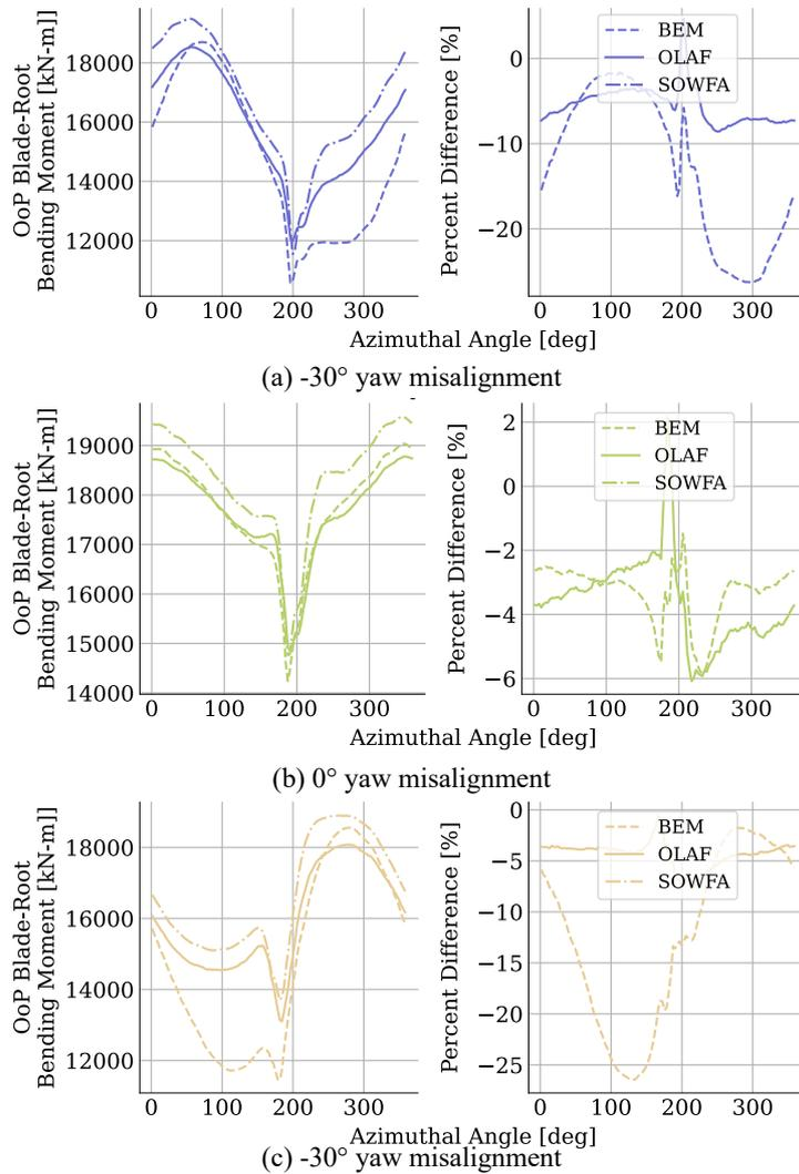
**Figure 7.** Azimuthal-averaged quantities for OLAF, BEM, and SOWFA results with varying yaw misalignment angles. Plots on the left show mean quantities, and plots on the right show percent difference of the means from SOWFA results. Line color indicates yaw misalignment angle, and line style indicates computational method. SOWFA results are shown as a dash-dot line, OLAF results are shown as solid lines, and BEM results are shown as dashed lines.
