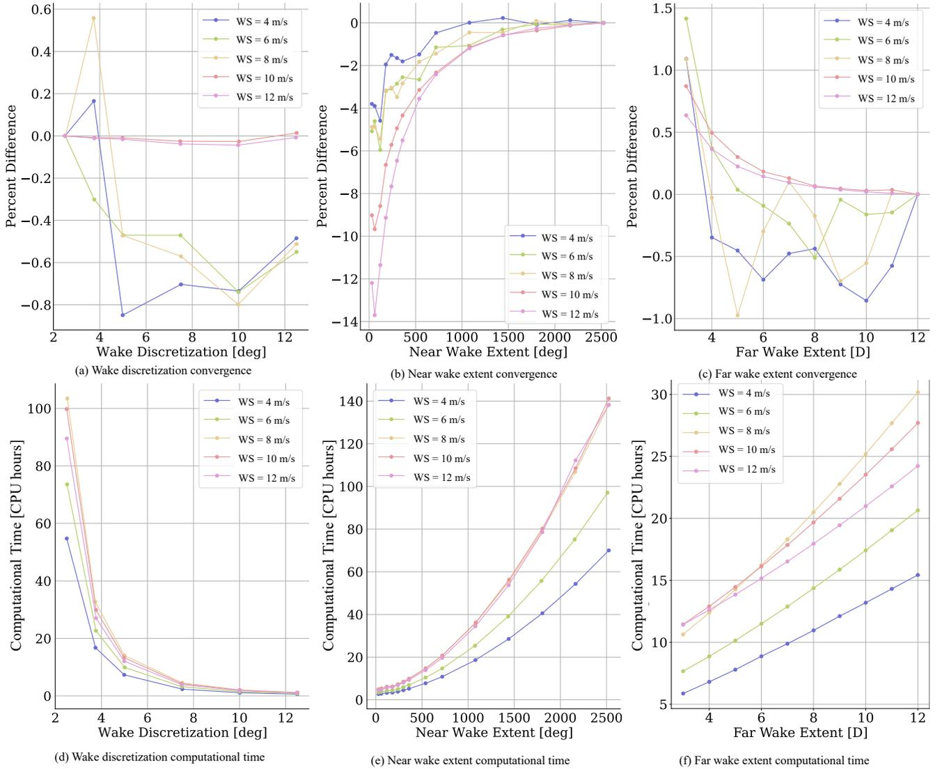
**Figure 2.** Percent differences (top) and computational time (bottom) of time-averaged rotor power, varying for (a, d) wake discretization, (b, e) near wake extent, and (c, f) far wake extent. Each line color represents a different hub-height wind speed. Wake discretization results are relative to  $2.5^\circ$ . Near wake extent results are relative to  $2520^\circ$  (7 revolutions). Far wake extent results are relative to 12D.
