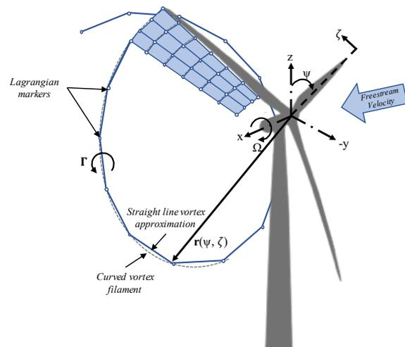
**Figure 1.** Evolution of near-wake lattice, blade tip vortex, and Lagrangian markers. Note that the blade root vortex is also present in the formulation, but not shown in the figure.
