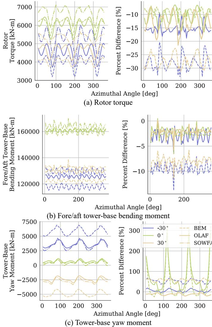
**Figure 8.** Azimuthal-averaged quantities for OLAF, BEM, and SOWFA results with varying yaw misalignment angles. Plots on the left show mean quantities, and plots on the right show percent difference of the means from SOWFA results. Line color indicates yaw misalignment angle, and line style indicates computational method. SOWFA results are shown as a dash-dot line, OLAF results are shown as solid lines, and BEM results are shown as dashed lines.
