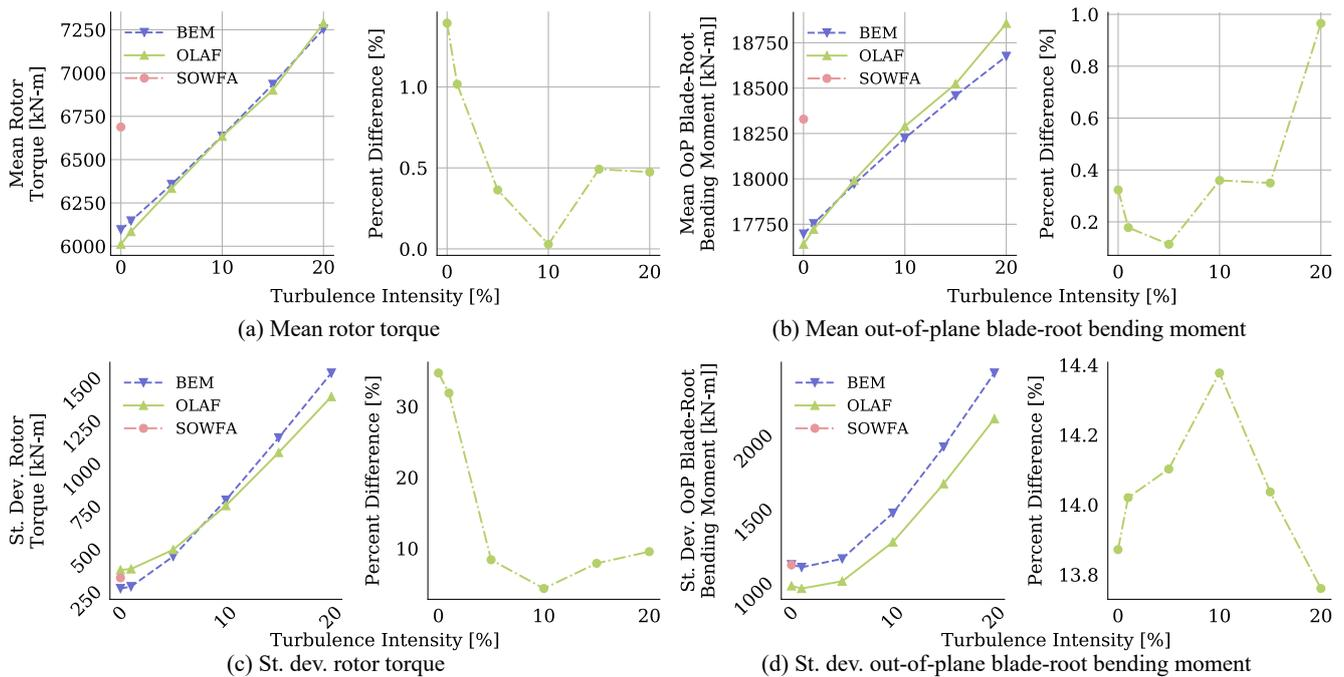
**Figure 13.** (a,b) Time-averaged and (c,d) standard deviation quantities for OLAF, BEM, and SOWFA results with varying inflow turbulence intensity. Plots on the left show mean quantities, and plots on the right show percent difference of the means from BEM results.
