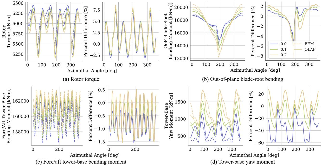
**Figure 12.** Azimuthal-averaged quantities for OLAF and BEM results with varying shear exponent. Plots on the left show mean quantities, and plots on the right show percent difference of the means from OLAF results. Line color indicates shear exponent, and line style indicates computational method. OLAF results are shown as solid lines and BEM results are shown as dashed lines.
