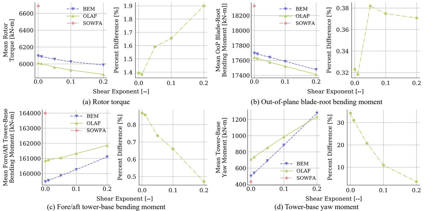
**Figure 10.** Time-averaged quantities for OLAF, BEM, and SOWFA results with varying shear exponent. Plots on the left show mean quantities and plots on the right show percent difference of the mean results.
