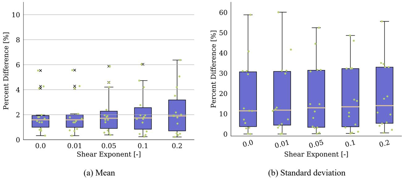
**Figure 11.** Average percent difference between BEM and OLAF results across all QoIs for varying inflow shear exponents. Each dot represents an individual QoI value (variation in  $x$ -axis location within a bar aids visualization). Box and whisker plots show the median (yellow line) value of all results; lower and upper quartile values (box edges); maximum and minimum values excluding outliers (whiskers); and outlier points ( $\times$  symbols), which also coincide with individual QoI values.
