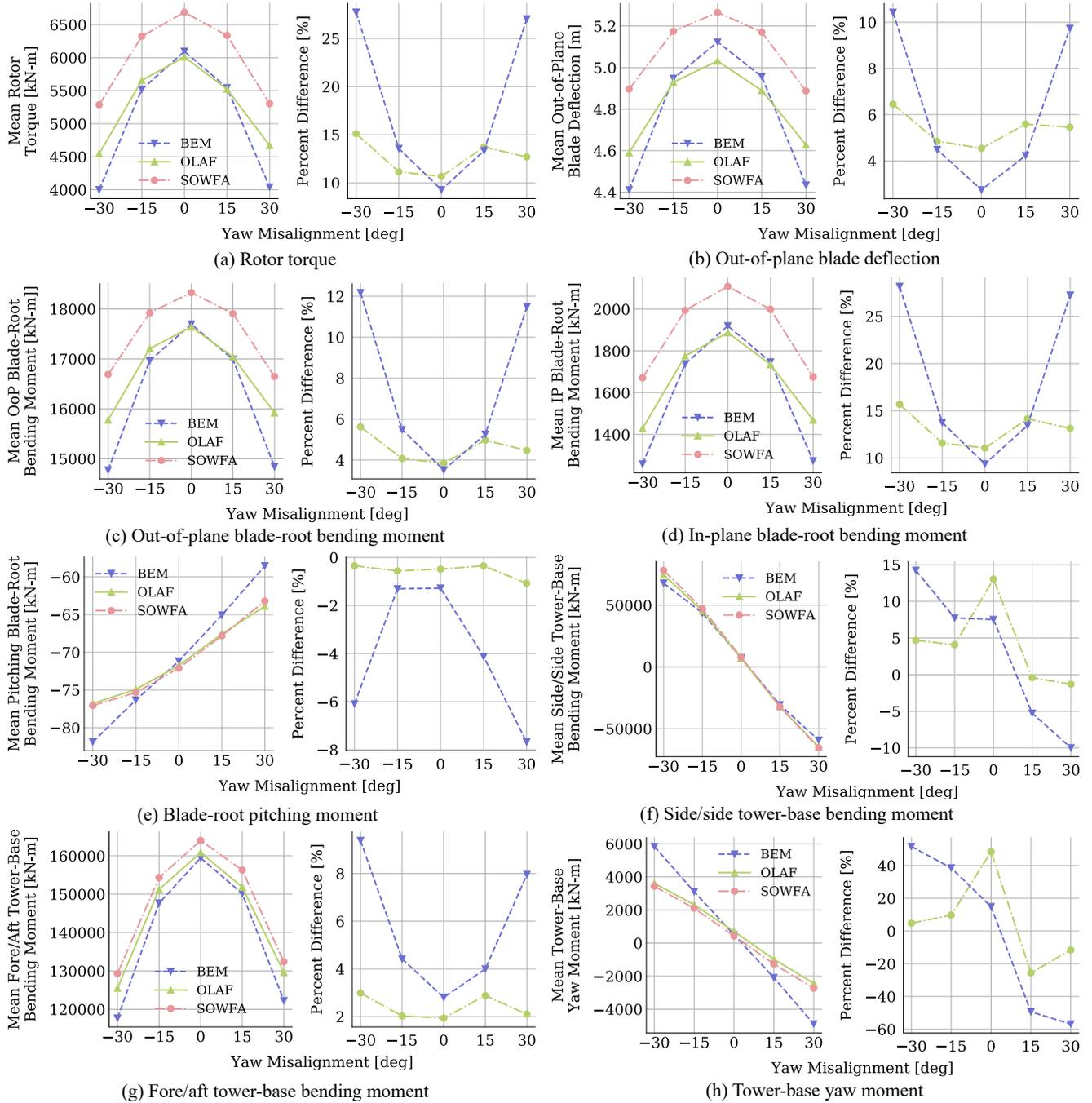
**Figure 5.** Time-averaged quantities for OLAF, BEM, and SOWFA results with varying yaw misalignment angles. Plots on the left show mean quantities and plots on the right show percent difference of the means from SOWFA results.
