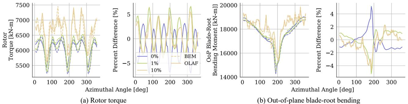
**Figure 15.** Azimuthal-averaged quantities for OLAF and BEM results with varying inflow turbulence intensity levels. Plots on the left show mean quantities and plots on the right show percent difference of the means from OLAF results. Line color indicates turbulence intensity level and line style indicates computational method. OLAF results are shown as solid lines and BEM results are shown as dashed lines.
