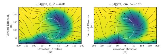
**Figure 7.** Time-averaged flow fields associated with the optimal power (left) and loading (right) found by the optimization, viewed from upstream, 6 rotor diameters (top) away from the front turbine, one rotor diameter upstream of the downstream turbine. Brighter colors indicate faster velocity magnitudes. In each plot, the vertical and crossflow location of the back turbine are shown as a white ellipse.
