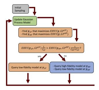
Figure 1. Workflow visualization for the bifidelity optimization case.  $\mathbf{h}^1$  is represented by  $GP^{\mathrm{LF}}$ ,  $\mathbf{h}^2$  is represented by  $GP^{\mathrm{HF}}$ ,  $C_1$  is represented by  $C_{\mathrm{LF}}$ , and  $C_2$  is represented by  $C_{\mathrm{HF}}$ .
