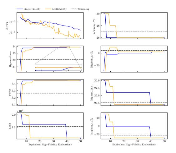
**Figure 3.** Convergence history of the single-fidelity and multifidelity approaches. The left plots show the EHVI, hypervolume, and best-observed power and loading. The right plots show the yaw configurations associated with the best-observed power and loading.
