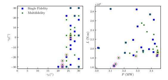
**Figure 4.** Sampled inputs and outputs associated with power greater than 3 MW and loads less than 3 MN-m. Points associated with the single-fidelity approach are shown using blue square markers, and points associated with the multifidelity approach are shown using green circular markers. A Pareto set constructed from the single-fidelity and multifidelity results is highlighted with hollow circles, where darker (magenta) circles correspond to Pareto points with lower loads and lower powers.
