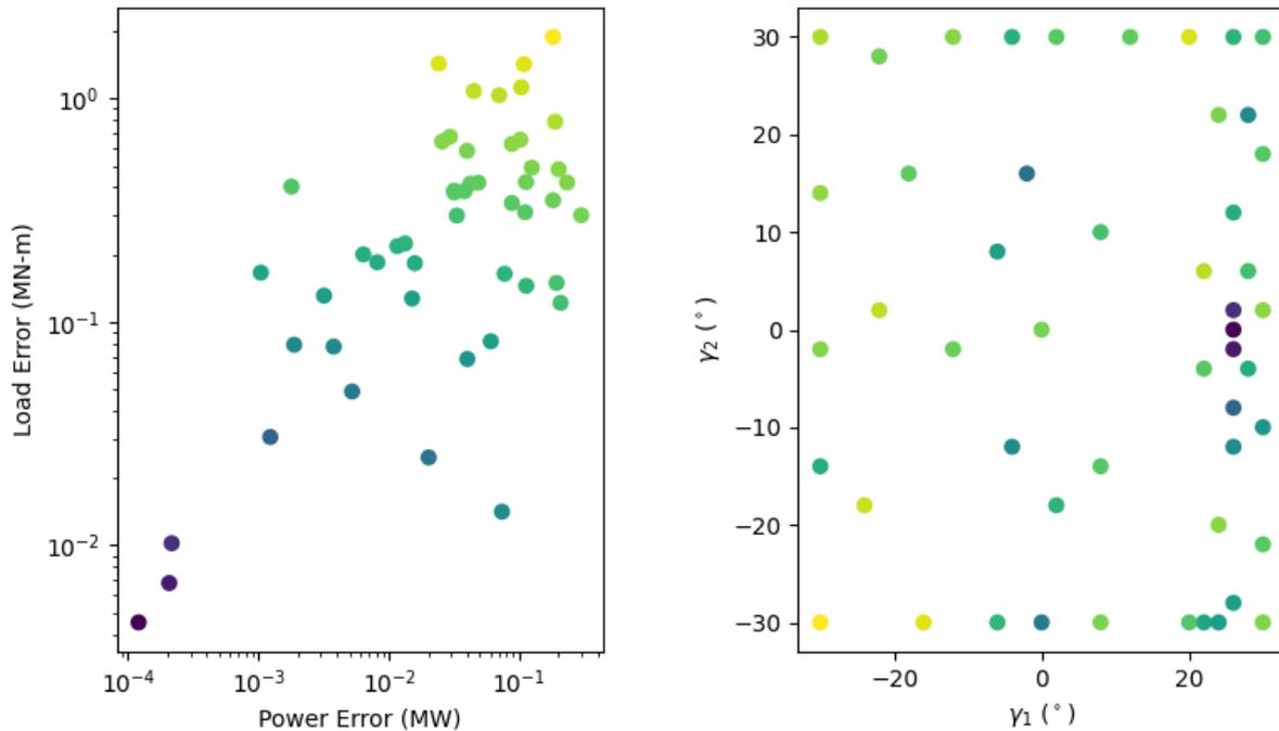
**Figure 9.** Results of the single-fidelity leave-one-out analysis. The left panel shows the leave-one-out prediction errors associated with power and loading, and the points are colored by the sum of both errors. The same points are plotted in the right panel, showing their associated  $\gamma_1$  and  $\gamma_2$  values.
