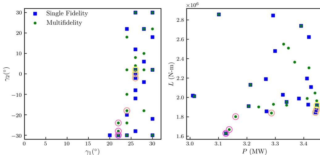
**Figure 4.** Sampled inputs and outputs associated with power greater than 3 MW and loads less than 3 MN-m. Points associated with the single-fidelity approach are shown using blue square markers, and points associated with the multifidelity approach are shown using green circular markers. A Pareto set constructed from the single-fidelity and multifidelity results is highlighted with hollow circles, where darker (magenta) circles correspond to Pareto points with lower loads and lower powers.
