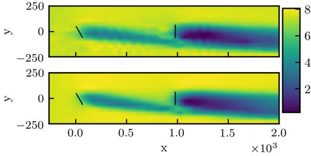
**Figure 2.** Time averaged velocity magnitude fields at the turbine hub height associated with the low- and high-fidelity models. The top panel shows the flow field associated with the low-fidelity model and the bottom panel shows the flow field associated with the high-fidelity model. In both cases, the front turbine is offset by  $30^\circ$  and the back turbine has no yaw offset. Brighter colors correspond to faster velocity magnitudes. Turbine positions are shown with dark lines.
