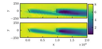
**Figure 2.** Time averaged velocity magnitude fields at the turbine hub height associated with the low- and high-fidelity models. The top panel shows the flow field associated with the low-fidelity model and the bottom panel shows the flow field associated with the high-fidelity model. In both cases, the front turbine is offset by  $30^{\circ}$  and the back turbine has no yaw offset. Brighter colors correspond to faster velocity magnitudes. Turbine positions are shown with dark lines.
