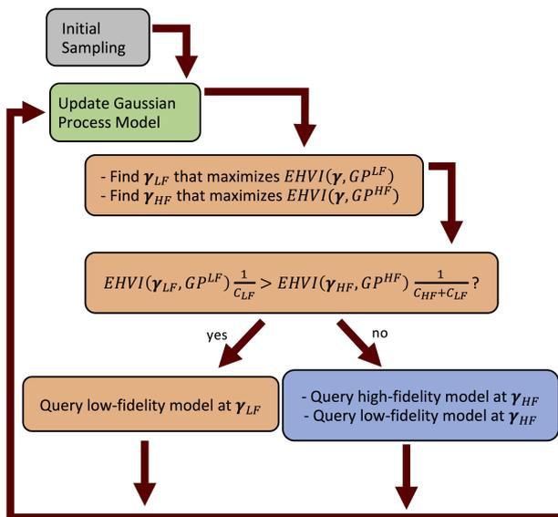
**Figure 1.** Workflow visualization for the bifidelity optimization case.  $\mathbf{h}^1$  is represented by  $GP^{LF}$ ,  $\mathbf{h}^2$  is represented by  $GP^{HF}$ ,  $C_1$  is represented by  $C_{LF}$ , and  $C_2$  is represented by  $C_{HF}$ .
