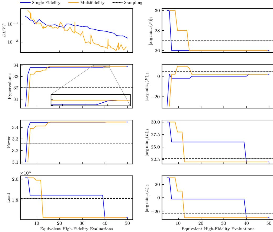
**Figure 3.** Convergence history of the single-fidelity and multifidelity approaches. The left plots show the EHV1, hypervolume, and best-observed power and loading. The right plots show the yaw configurations associated with the best-observed power and loading.
