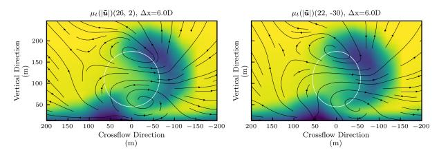
**Figure 7.** Time-averaged flow fields associated with the optimal power (left) and loading (right) found by the optimization, viewed from upstream, 6 rotor diameters (top) away from the front turbine, one rotor diameter upstream of the downstream turbine. Brighter colors indicate faster velocity magnitudes. In each plot, the vertical and crossflow location of the back turbine are shown as a white ellipse.
