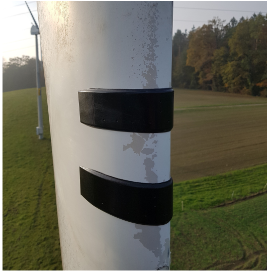
Figure 5. 3D polyjet printing housings glued on an operating 6 kW operating wind turbine to test its robustness
