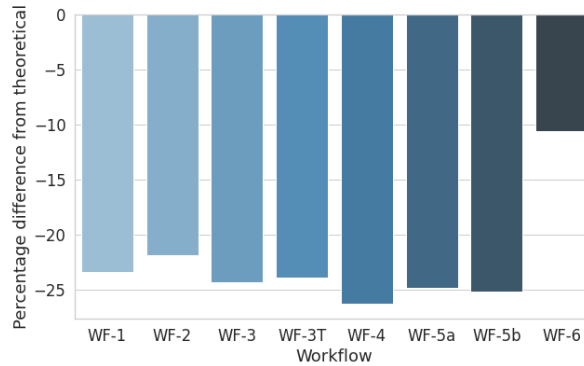
Figure 11. Site 1 - Percentage difference in gross AEP from the 'theoretical' value for each workflow applied
