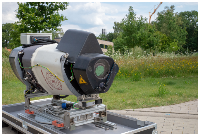
Figure 1. The SpinnerLidar with its mounting platform at ForWind - University of Oldenburg.
