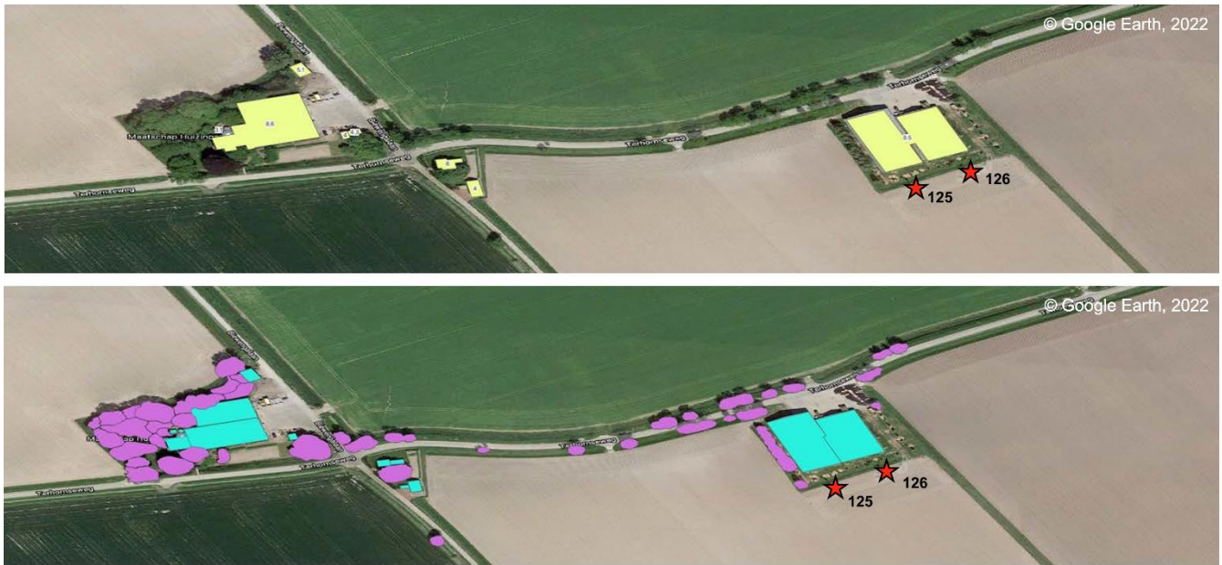
Figure 3. (a; Top) Obstacle annotations for a site with two turbines using data commercially available from 3dBuildings.com (b; Bottom) Full annotations using semi-automated annotation process including both buildings and vegetation, enriched with lidar data.
