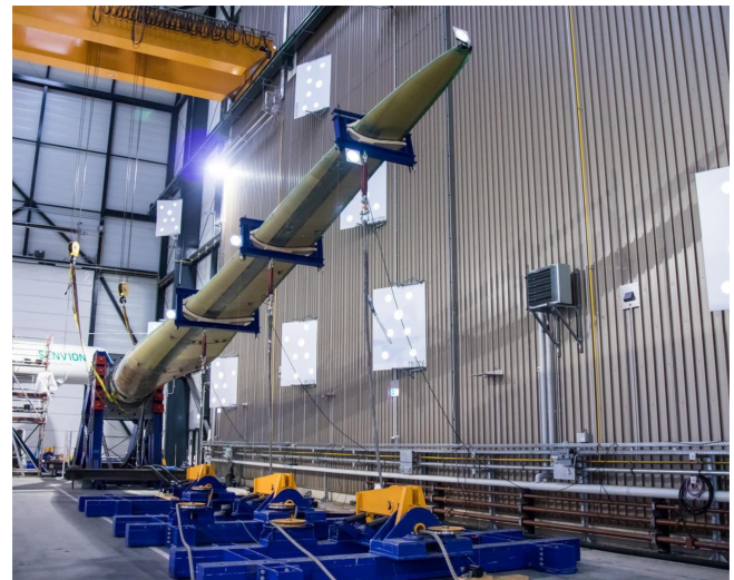
Figure 8. Photo of a static blade test configuration in flapwise direction.
