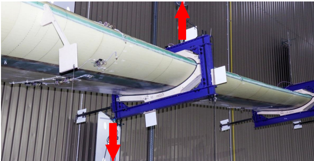
Figure 9. Configuration example of a static torsional loading on the blade with marked up and downwards facing forces.
