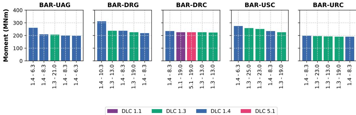
**Figure 4.** Ranking of the fore-aft moments at tower base for the BAR designs. The colors represent the different design load cases (DLCs) listed in Table 5. The moments do not include partial safety factors.
