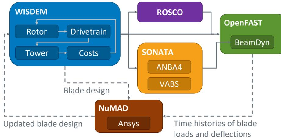
**Figure 1.** Scheme illustrating the sequence of numerical frameworks adopted in this study. WISDEM is described in Sect. 2; and ROSCO, SONATA, and OpenFAST are described in Sect. 3. NuMAD and the data flow to it, which is represented by the dashed line, are described in Camarena et al. (Under Submission at the Journal of Wind Energy Science).
