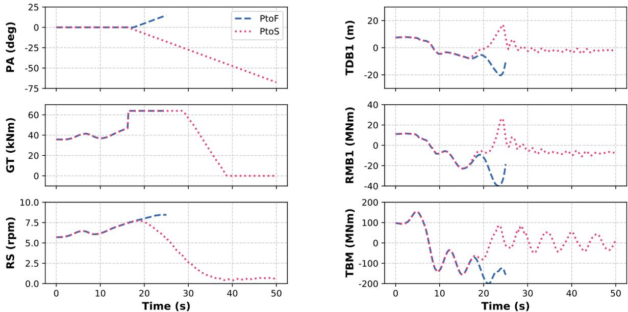
**Figure 5.** Comparison of the time histories of pitch angle (PA) in deg, generator torque (GT) in kNm, rotor speed (RS) in revolutions per minute, flapwise tip deflection of Blade 1 (TDB1) in m, flapwise root moment of Blade 1 (RMB1) in MNm, and fore-aft tower base moment (TBM) in MNm for the pitch-to-feather (PtoF) and pitch-to-stall (PtoS) for the BAR-DRC design during an extreme gust with change of direction. PtoF is interrupted at 25 s because of a tower-strike event of Blade 2.
