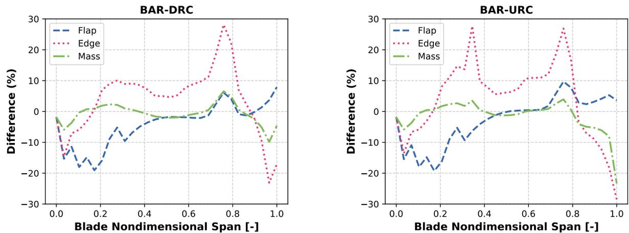
**Figure 2.** Difference in flapwise stiffness, edgewise stiffness, and unit mass distributions between PreComp and ANBA4 for the designs BAR-DRC and BAR-URC. Negative values mean that ANBA4 predicts lower values than PreComp.
