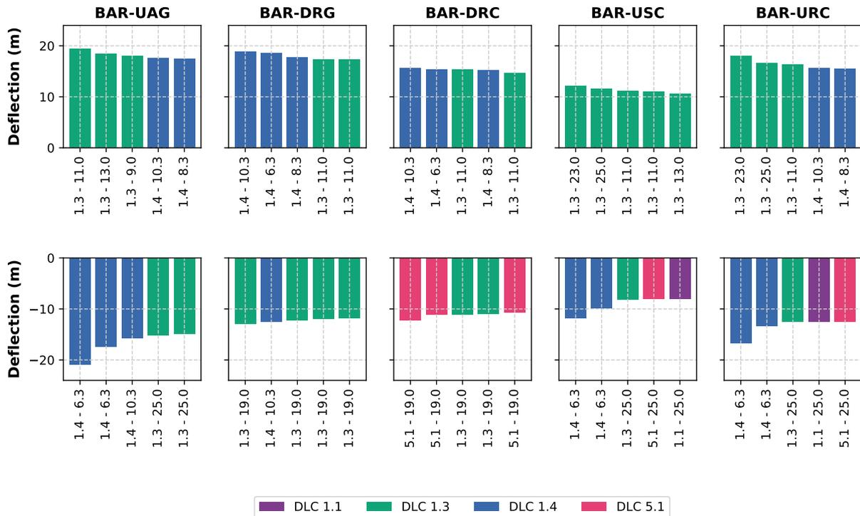
**Figure 3.** Ranking of the out-of-plane blade deflections for the BAR designs. Deflections are aligned with the primary wind direction, so deflections toward the tower are positive in upwind rotors (BAR-UAG, BAR-USC, and BAR-URC) and negative in downwind rotors (BAR-DRG and BAR-DRC). The colors represent the different design load cases (DLCs) listed in Table 5. The deflections do not include partial safety factors.
