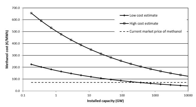
Figure 8 Cost of methanol produced by FARWIND systems as function of the installed capacity and comparison with the current market price of methanol produced from fossil fuels and fossil feedstocks.
