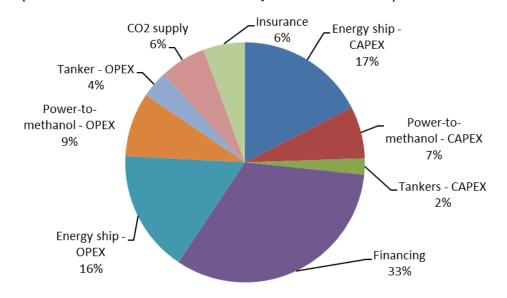
Figure 7 Cost breakdown of methanol produced by a first-of-a-kind FARWIND system. The shown data corresponds to an average cost scenario (methanol cost equal to 2.4 €/kg).
