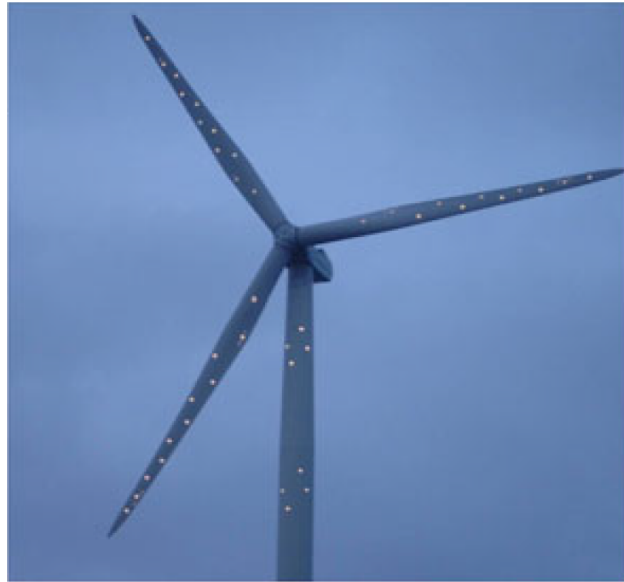
Figure 6. Example of turbine instrumentation with reflective markers for photogrammetry or laser interferometry (Ozbek and Rixen, 2013).
