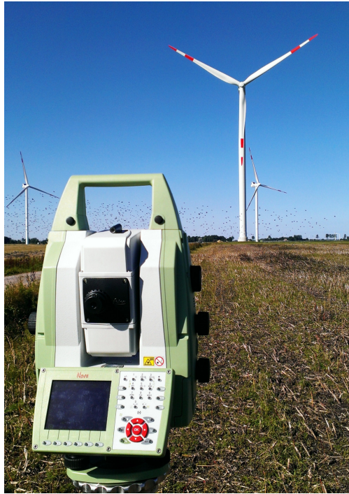
Figure 1. Measurement setup: tachymeter and turbine at a standstill.
