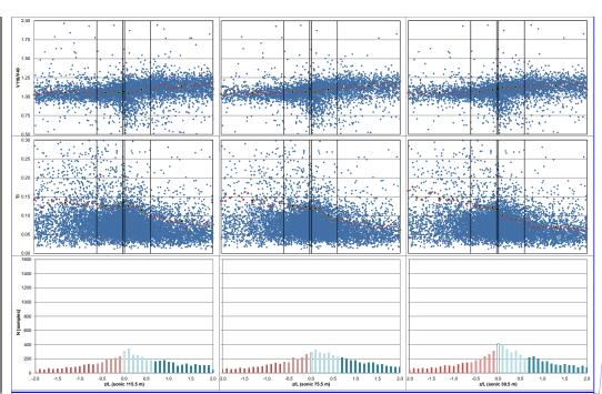
Figure 10 Wind shear and turbulence intensity vs sonic stability in MP5, [157.5°-202.5°] sector. Red dots are the z/L mean values for 0.01 resolution scale, black squares are the z/L mean values in each of the stability classes according to Table 1.
