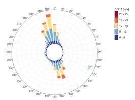
Figure 2 Wind rose of 10 min wind speeds observed by MP5 at 118m for the reference period (July 2014–June 2015).
