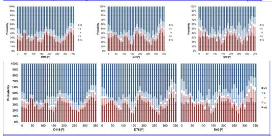
Figure 8 Distribution of atmospheric stability with wind direction based on z/L obtained with sonic anemometer at different heights. vs, very stable; s, stable; n, neutral; u, unstable; vu, very unstable.
