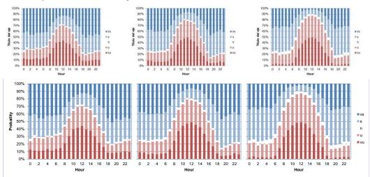
Figure 6 Distribution of atmospheric stability with hour based on z/L obtained with sonic anemometer at different heights, left 115.5 m, center 75.5m and right 39.5 m. vs, very stable; s, stable; n, neutral; u, unstable; vu, very unstable.
