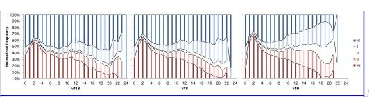
Figure 5 Distribution of atmospheric stability with wind speed based on z/L obtained with sonic anemometer at different heights, 115.5 m on the left, 75.5 m in the middle and 39.5 m on the right side. vs, very stable; s, stable; n, neutral; u, unstable; vu, very unstable.
