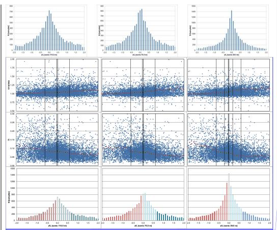
Figure 9 Wind shear and turbulence intensity vs sonic stability in MP5, [337.5°-22.5°] sector. Red dots are the z/L mean values for 0.01 resolution scale, black squares are the z/L mean values in each of the stability classes according to Table 1.
