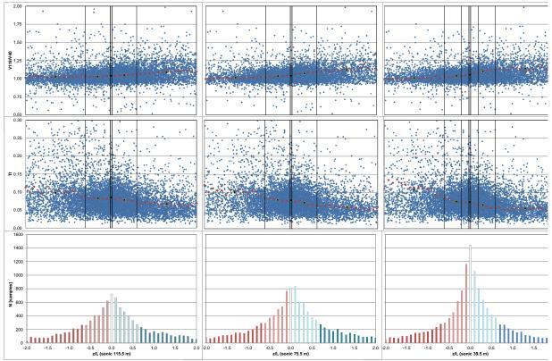
Wind shear and turbulence intensity vs sonic stability in MP5, [337.5°-22.5°] sector. Red dots are the z/L mean Figure 9 for 0.01 resolution scale, black squares are the z/L mean values in each of the stability classes according to Table 1.
