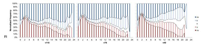
Distribution of atmospheric stability with wind speed based on z/L obtained with sonic anemometer at different heights, 115.5 m on the left, 75.5 m in the middle and 39.5 m on the right side. vs, very stable; s, stable; n, neutral; u, unstable; vu, very unstable.
