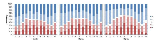
Figure 7 Monthly distribution of stability based on z/L obtained with sonic anemometer at different heights, left 115.5 m, center 75.5 m and right 39.5 m. vs, very stable; s, stable; n, neutral; u, unstable; vu, very unstable.
