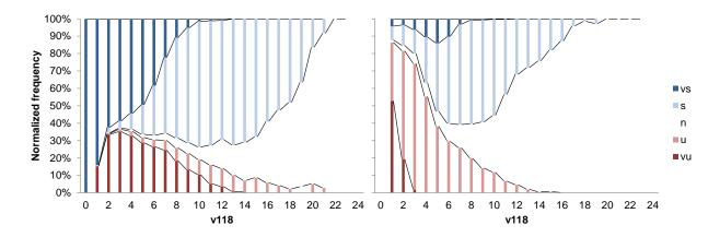
Figure 12 Distribution of atmospheric stability with wind speed. On the left based on  $Ri_b$ ; On the right based on z/L obtained from  $Ri_b$  with transformation functions by Businger and Dyer. vs, very stable; s, stable; n, neutral; u, unstable; vu, very unstable.
