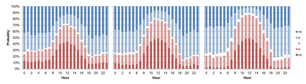
Distribution of atmospheric stability with hour based on z/L obtained with sonic anemometer at different heights, left 115.5 m, center 75.5m and right 39.5 m. vs, very stable; s, stable; n, neutral; u, unstable; vu, very unstable.
