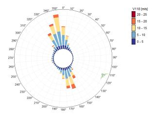
Wind rose of 10 min wind speeds observed by MP5 at 118m for the reference period (July 2014-June 2015).
