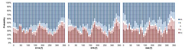
Distribution of atmospheric stability with wind direction based on z/L obtained with sonic anemometer at different heights. vs, very stable; s, stable; n, neutral; u, unstable; vu, very unstable.
