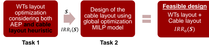
Figure 5. Approach 2: Simultaneous design process for WTs and cable layout.
