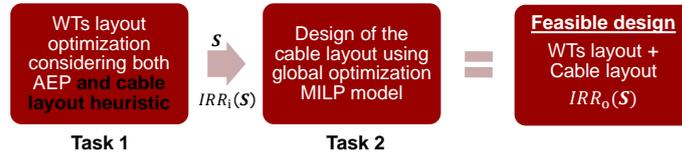
Figure 5. Approach 2: Simultaneous design process for WT and cable layout.
