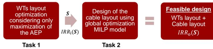
Figure 4. Approach 1: Sequential design process for WT and cable layout.
