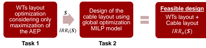
Figure 4. Approach 1: Sequential design process for WTs and cable layout.
