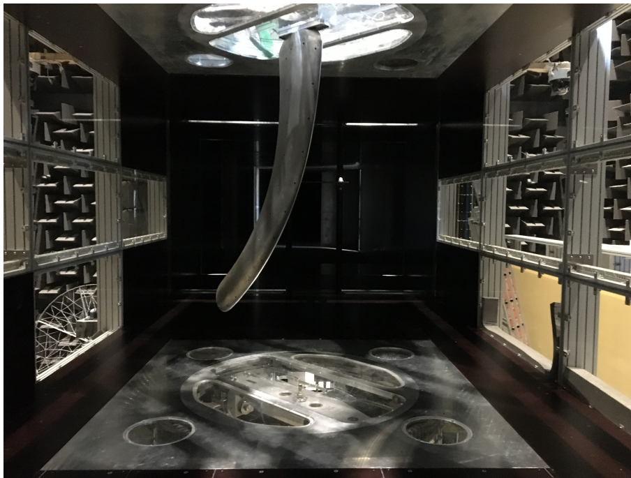
Figure 6. The tip model mounted in the test section of the Poul la Cour wind tunnel.
