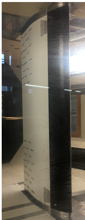
Figure 6. Example of tuft visualisation obtained for a clean airfoil (i.e. no tripping) with a slat at Re = 1.5 \cdot 10^6 and a small angle of attack.
