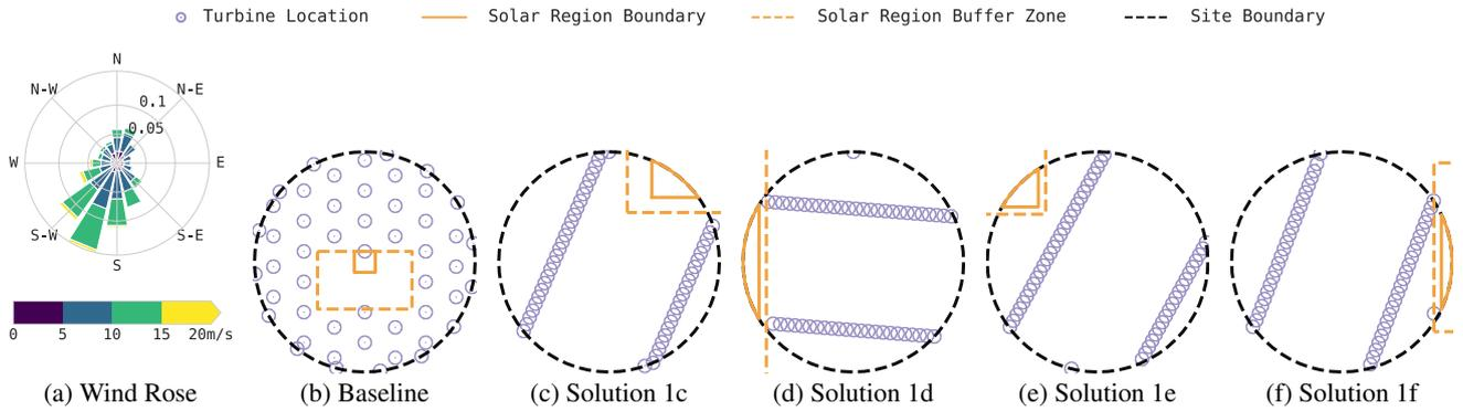
**Figure 1.** CMA-ES solutions for the high-correlation location and circular boundary. Turbine locations are marked in purple, the solar region is drawn with an orange solid line, and the surrounding solar buffer zone is marked with a dashed orange line.
