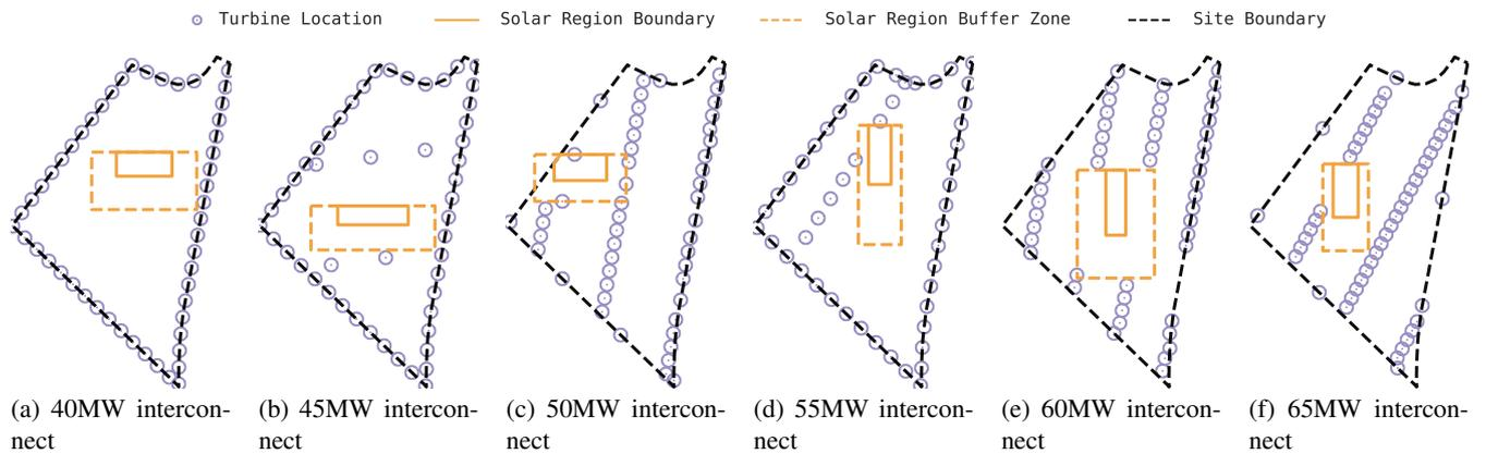
**Figure 3.** Solutions generated for the high-correlation location and irregular boundary for a range of interconnect capacities, maximizing mean interconnect utilization instead of AEP.
