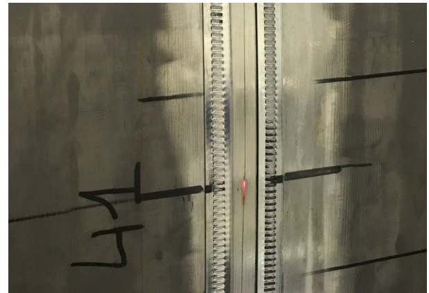
Figure 5. Detail view of an optical fiber where a Bragg grating is illuminated in red (S41).
