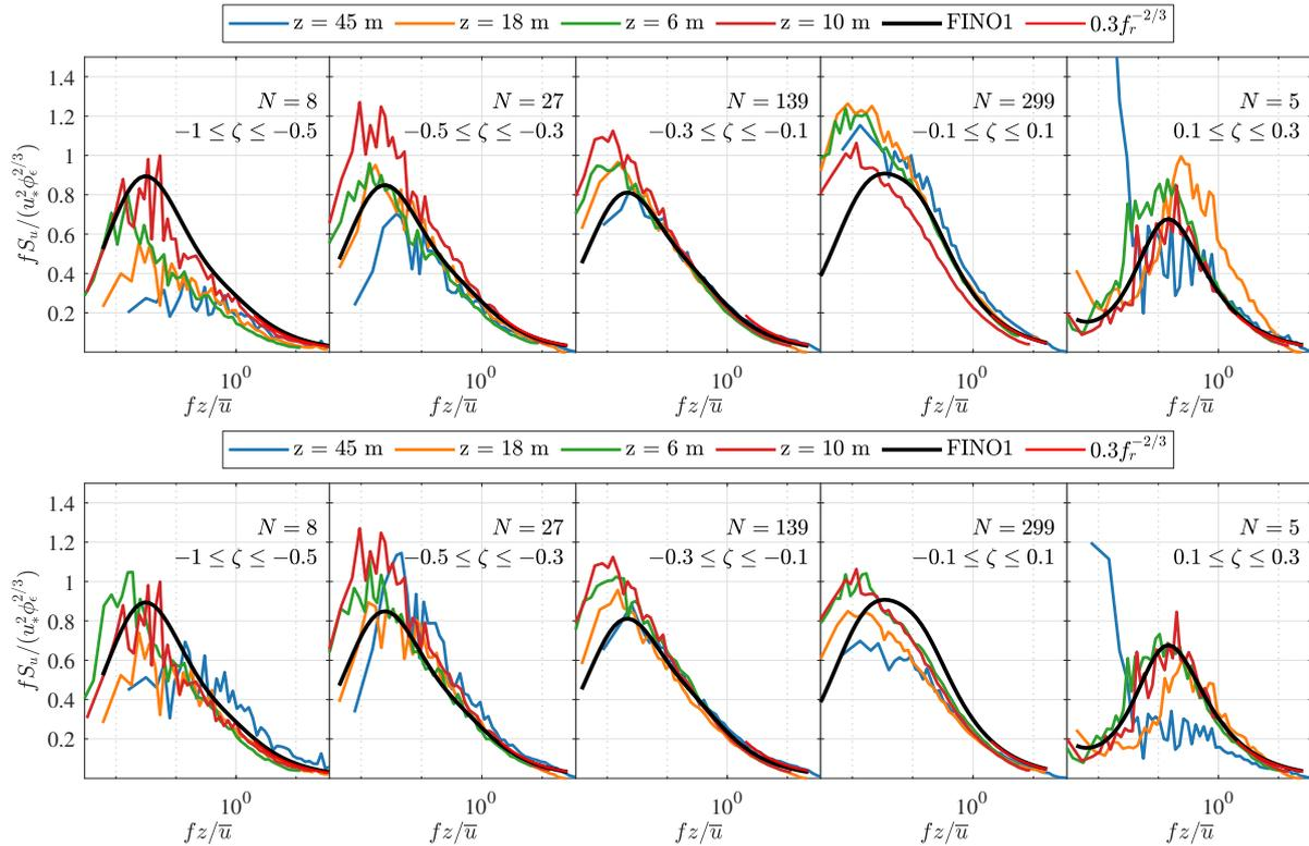
Figure 3: Power spectral densities of the along-wind component using the uncorrected friction velocity (top panels) and corrected one (bottom panels). The parameter  $z/L$  was estimated at 10 m and the data set relied on measurements from May 1994 to September 1994.
