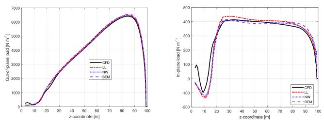
**Figure 8.** Comparison of out-of-plane load (left) and in-plane load (right) of the baseline straight blade calculated from the Navier-Stokes solver (CFD), the lifting-line method (LL), the proposed coupled method (NW) and the blade element momentum method (BEM).
