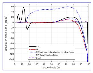
**Figure C4.** Comparison of the difference between the out-of-plane load (left) and the in-plane load (right) of the forward swept Blade-6 with respect to the baseline blade calculated from the Navier-Stokes solver (CFD), the lifting-line method (LL), the proposed coupled method (NW) and the blade element momentum method (BEM).
