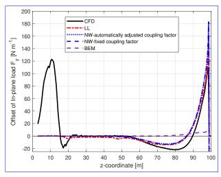
**Figure C1.** Comparison of the difference between the out-of-plane load (left) and the in-plane load (right) of the backward swept Blade-2 with respect to the baseline blade calculated from the Navier-Stokes solver (CFD), the lifting-line method (LL), the proposed coupled method (NW) and the blade element momentum method (BEM).
