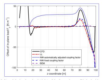
**Figure C5.** Comparison of the difference between the out-of-plane load (left) and the in-plane load (right) of the forward swept Blade-6 with respect to the baseline blade calculated from the Navier-Stokes solver (CFD), the lifting-line method (LL), the proposed coupled method (NW) and the blade element momentum method (BEM).
