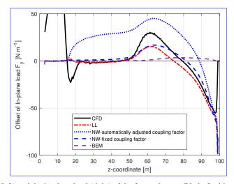
**Figure 10.** Comparison of the difference between the out-of-plane load (left) and the in-plane load (right) of the forward swept Blade-5 with respect to the baseline blade calculated from the Navier-Stokes solver (CFD), the lifting-line method (LL), the proposed coupled method (NW) and the blade element momentum method (BEM).
