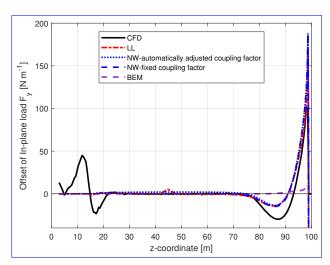
**Figure C3.** Comparison of the difference between the out-of-plane load (left) and the in-plane load (right) of the backward swept Blade-4 with respect to the baseline blade calculated from the Navier-Stokes solver (CFD), the lifting-line method (LL), the proposed coupled method (NW) and the blade element momentum method (BEM).
