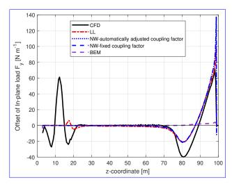
**Figure C2.** Comparison of the difference between the out-of-plane load (left) and the in-plane load (right) of the backward swept Blade-3 with respect to the baseline blade calculated from the Navier-Stokes solver (CFD), the lifting-line method (LL), the proposed coupled method (NW) and the blade element momentum method (BEM).
