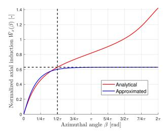
Figure 3. Illustration of the difference between the analytical and the approximated normalized trailing functions (left) and the corresponding induction functions (right). The parameters for the illustration are h/r=0.5,  $\psi=10^\circ$ ,  $\varphi=5^\circ$ . The approximated steady-state near-wake induction is when  $\beta=\infty$  and corresponds to the analytical near-wake induction at  $\beta=\frac{\pi}{2}$ .
