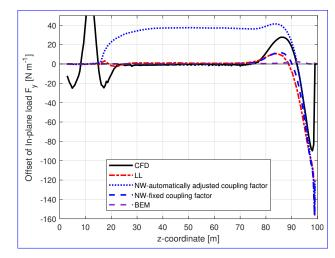
**Figure C6.** Comparison of the difference between the out-of-plane load (left) and the in-plane load (right) of the forward swept Blade-8 with respect to the baseline blade calculated from the Navier-Stokes solver (CFD), the lifting-line method (LL), the proposed coupled method (NW) and the blade element momentum method (BEM).
