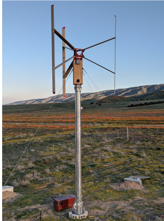
Figure 9. Photo of XFlow’s 5-kW prototype VAWT at the Field Laboratory for Optimized Wind Energy in Lancaster, CA California.
