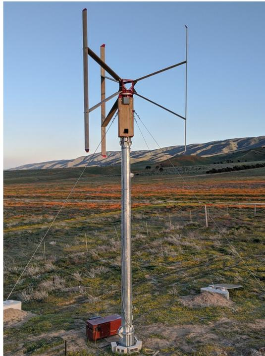
**Figure 8.** Photo of XFlow’s 5-kW prototype VAWT at the Field Laboratory for Optimized Wind Energy in Lancaster, CA
