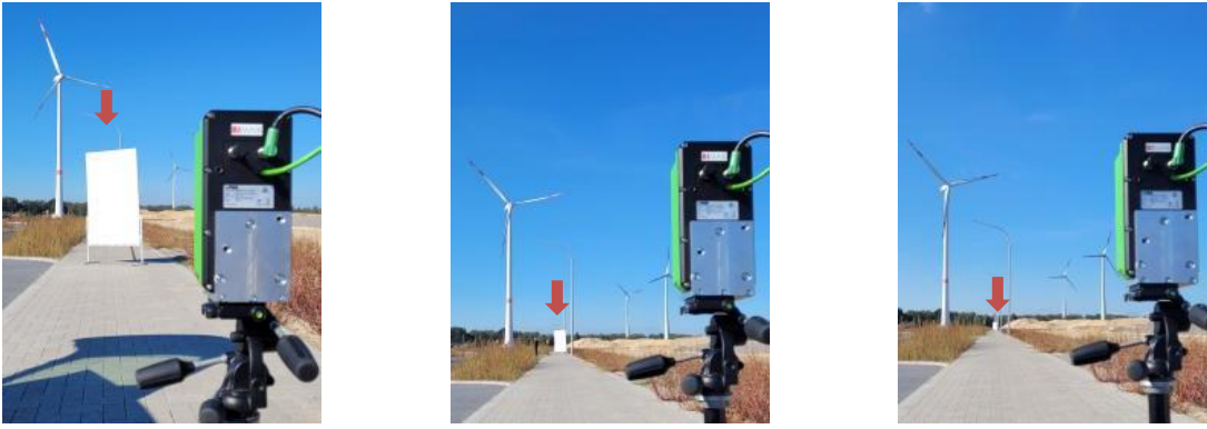
Figure 4: White board (marked with red arrow) placed at different working distances and with different angles with respect to the laser scanner. The number of scans for each position and orientation amounts to > 10,000 .
