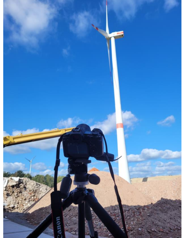
Figure 3: Left: experimental setup for field measurements with a laser scanner on a tripod, a measurement laptop and the wind turbine in the background. Right: experimental setup for field measurement with a camera on a tripod and the wind turbine from the side in the background used as a reference for the tower-blade tip clearance.
