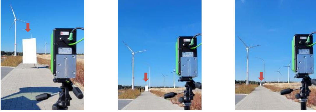
200 Figure 4: White board (marked with red arrow) placed at different working distances and with different angles with respect to the laser scanner. The number of scans for each position and orientation amounts to > 10,000 .
