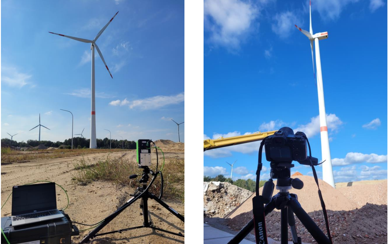
Figure 3: Left: experimental setup for field measurements with a laser scanner on a tripod, a measurement laptop and the wind turbine in the background. Right: experimental setup for field measurement with a camera on a tripod and the wind turbine from the side in the background used as a reference for the tower-blade tip clearance.
