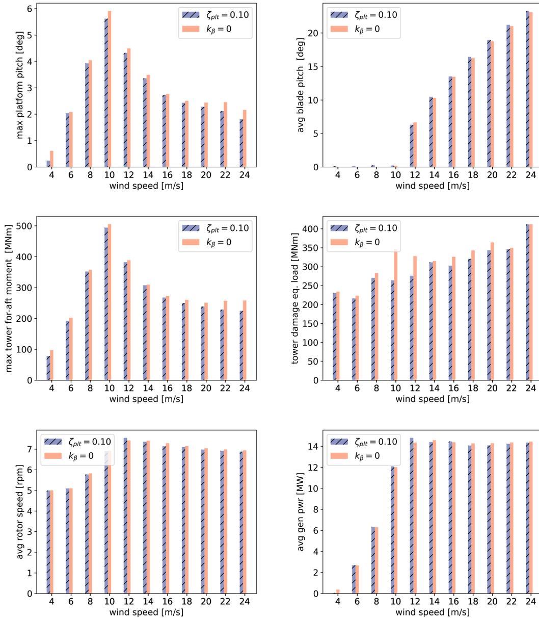
**Figure 13.** Comparison results for the DLC1.2 for the UMaine floater with IEA15MW WTG. The imposed level of damping in the platform dynamics for the  $\zeta_{plt}$ -fixed strategy is 0.10. Outputs show statistics for platform pitch; blade pitch; Tower bending moment, max and damage equivalent load; rotor speed and generator power.
