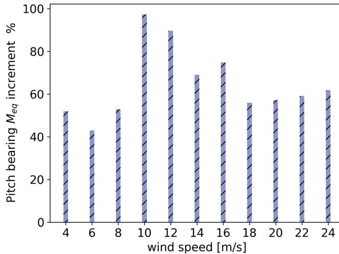
**Figure 15.** Increment in the use of the pitch bearing given by the  $\zeta_{plt}$ -fixed strategy with respect to the reference. The increment is expressed in terms of % of  $M_{eq}$  (eq. 53)
