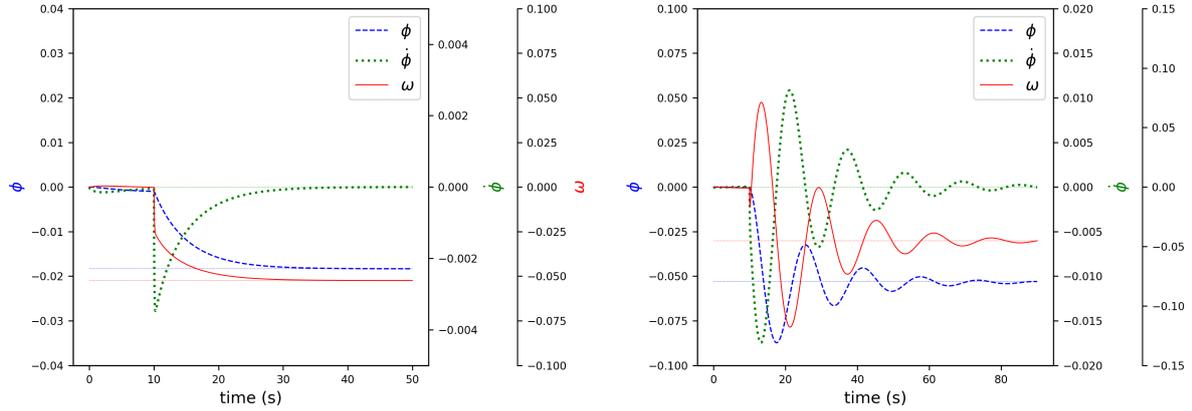
**Figure 3.**  $\omega$  responses to a  $\beta$ -step input (at  $t = 10s$ ). On the left, parameters (Table 2) are chosen so that the condition eq. 28 is false:  $\omega$  decreases. On the right, parameters are chosen so that condition eq. 28 is true: at first  $\omega$  increases even though  $\beta$  has step up.
