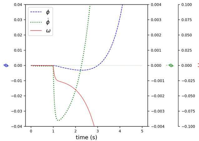
**Figure 4.** hypothetical situation where both conditions eq. 25 and eq. 28 are true. At first, both  $\phi$  and  $\omega$  decrease, but soon they both diverge because of the negative damping ( $k_P/k_I$  corrections can delay this divergence but can not avoid it).
