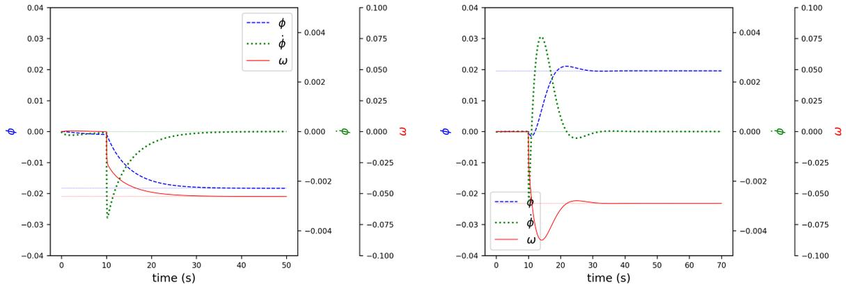
**Figure 2.**  $\phi$  and  $\omega$  responses to a  $\beta$ -step input (at  $t = 10$ s): on the left, values (Table 1) are chosen so that eq. 25 is false:  $\phi$  decreases. On the right, values (Table 1) are chosen so that the eq. 25 is true:  $\phi$  increases even though  $\beta$  has step up.
