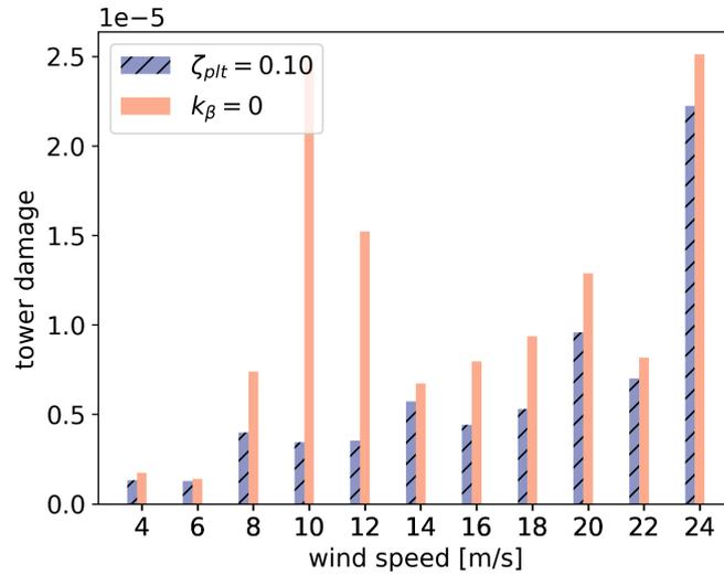
**Figure 14.** Fatigue cumulative damage at tower bottom by using rainflow counting and linear Miner’s rule. The damage is obtained considering the tower base design proposed by the UMaine, a Wohler’s curve bi-linear with  $m = 3.0$  up to  $10^6$  cycles and  $m = 5.0$  after, as proposed by DNV for Offshore steel. The probability of occurrence of each wind is equal, without any weibull distribution.
