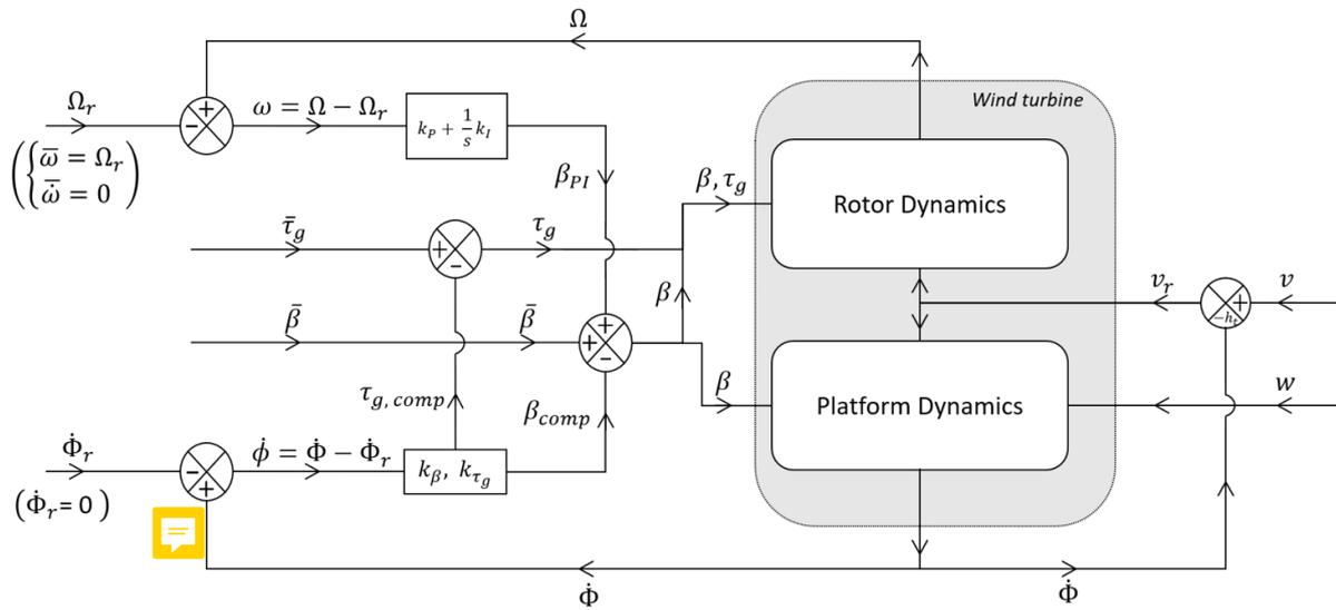
**Figure 1.** Block diagram of the controller model
