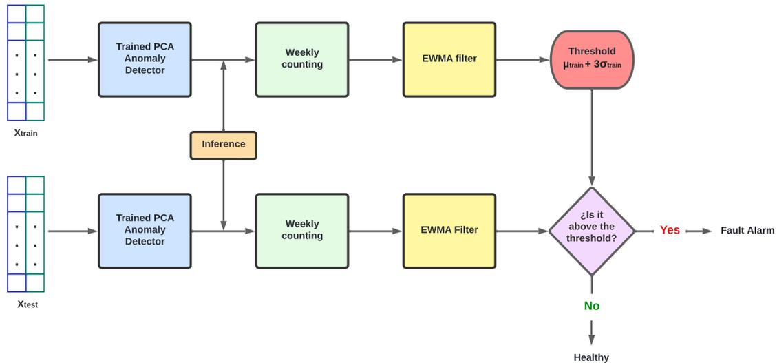
**Figure 10.** Second phase of the stated methodology.
