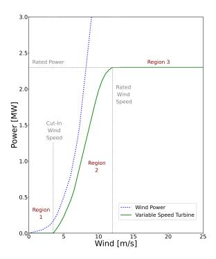
Figure 1. Wind turbines calculated power curve.
