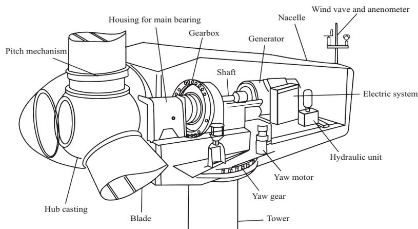
**Figure 2.** Main components of WTs. (Jiang et al., 2017).
