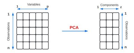
Figure 7. Dimensionality reduction applying PCA.
