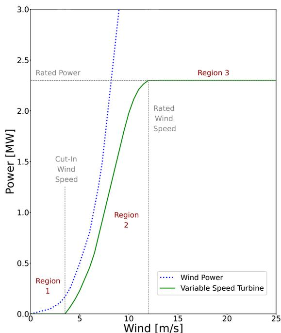
**Figure 1.** Wind turbines calculated power curve.
