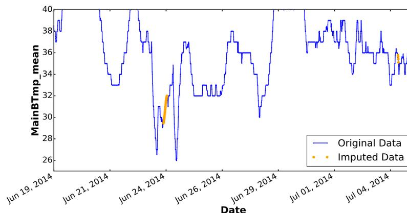
**Figure 5.** Imputation strategy used to fill missing values in the low-speed shaft temperature.
